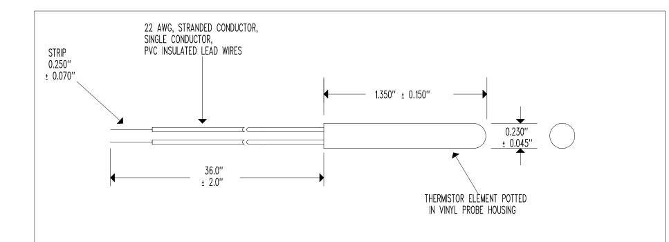
RESISTANCE @  $+25^{\circ}\text{C} = 10,000 \ \Omega \pm 1\%$ RESISTANCE/TEMPERATURE CURVE = "J" TEMPERATURE COEFFICIENT @  $+25^{\circ}\text{C} = -4.4\%$ /°C NOMINAL BETA " $\beta$ " (0 TO  $+50^{\circ}\text{C}$ ) = 3,892°K NOMINAL MAXIMUM TEMPERATURE RATING =  $+80^{\circ}\text{C}$
