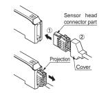
Note: Take care that if the connector is pulled out without pressing the projection, the projection may break. Do not use a sensor head connector whose projection has broken. Furthermore, do not pull by holding the cable, as this can cause a cable-break.
