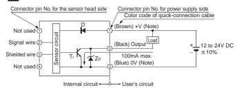
Note: The quick-connection cable does not have +V(Blown) and 0V(Blue). The supply voltage is supplied through the main cable connector.
