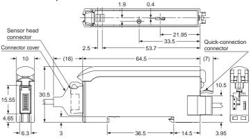
Note: The side view is with the sensor head connector and the quick-connection cable.
