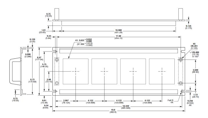
Accommodates up to four MP-2000 Readout/Controllers Dimensions are in inch (mm)
