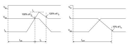
(a) Turn-on (b) Turn-off Figure 4. Switching Time Definitions
