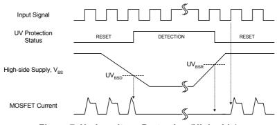
Figure 7. Undervoltage Protection (High-side)
