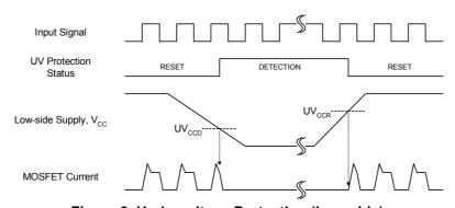
Figure 6. Undervoltage Protection (Low-side)
