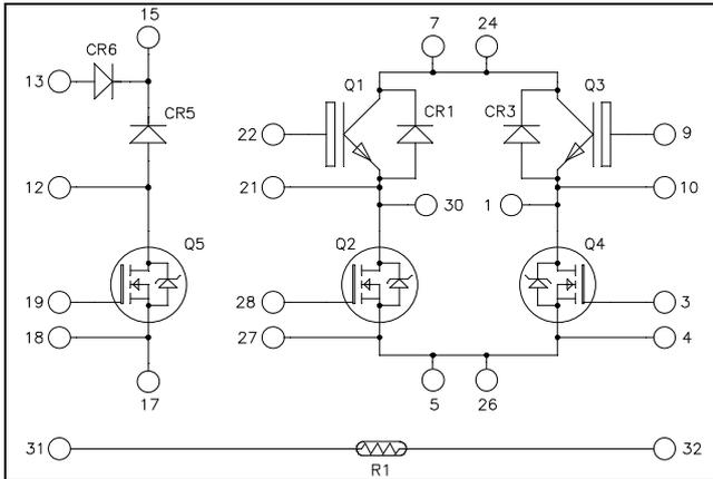
Top switches : Trench + Field Stop IGBT3
