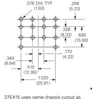
**Screw Terminal Socket For 4 Pole Relays**
