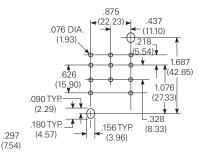
27E046 HAS TERMINALS .144" (3.66 mm) LONG. 27E305 HAS TERMINALS .184" (4.67 mm) LONG. 27E310 HAS TERMINALS .247" (6.27 mm) LONG.
