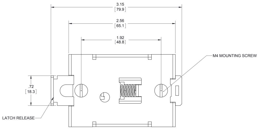
Tolerances: ± 0.02 in / 0.5 mm. All dimensions are in: inches [millimeters]
