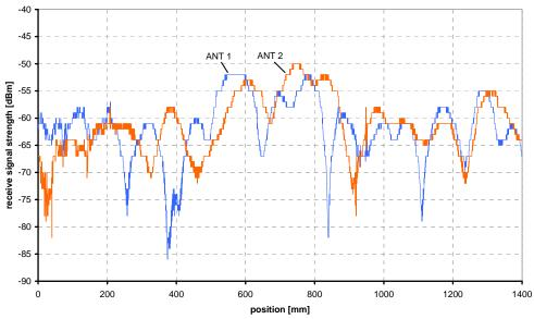
For a given position inside a network scenario with multipath fading effects, both antennas differ in their receive level (see **Figure 3-1**). This affects the packet error rate for small receive levels. Switching between both antennas and selecting the one that receives better can increase the reliability of a connection. For a detailed analysis see [3].
