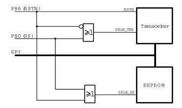
The EEPROM data is written during board production test. A unique serial number, the MAC address as well as calibration values are stored. These can be used to optimize system performance. The following table gives the data structure of the EEPROM.
