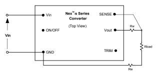
Fig. B: Remote sense circuit configuration.
