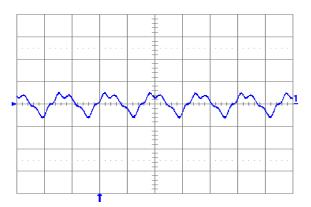
Fig. 3.3V.5: Output voltage ripple (20 mV/div.) at full rated load current into a resistive load with external capacitance 100 μF ceramic + 1μF ceramic and Vin = 12 V for Vout = 3.3 V. Time scale: 2 μs/div.
