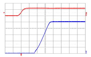
Fig. 5.0V.4: Turn-on transient for Vout = 5.0 V with application of Vin at full rated load current (resistive) and 100 µF external capacitance at Vin = 12 V. Top trace: Vin (10 V/div.); Bottom trace: output voltage (1 V/div.); Time scale: 2ms/div.
