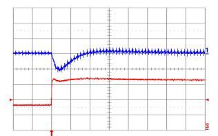
Fig. 1.5V.6: Output voltage response for Vout = 1.5V to positive load current step change from 8 A to 16 A with slew rate of 5 A/µs at Vin = 12 V. Top trace: output voltage (200 mV/div.); Bottom trace: load current (5 A/div.). Co = 100  $\mu$ F ceramic. Time scale: 20 µs/div.
