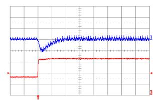
Fig. 5.0V.6: Output voltage response for Vout = 5.0 V to positive load current step change from 8 A to 16 A with slew rate of 5A/µs at Vin = 12 V. Top trace: output voltage (200 mV/div.); Bottom trace: load current (5A/div.). Co = 100  $\mu$ F ceramic. Time scale: 20 µs/div.
