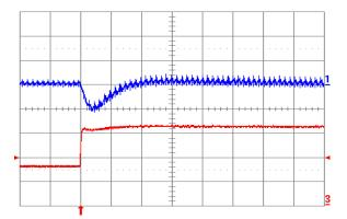
Fig. 2.5V.6: Output voltage response for Vout = 2.5 V to positive load current step change from 8 A to 16 A with slew rate of 5 A/ $\mu$ s at Vin = 12 V. Top trace: output voltage (200 mV/div.); Bottom trace: load current (5 A/div.). Co = 100  $\mu$ F ceramic. Time scale: 20 µs/div.
