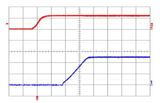
Fig. 2.5V.4: Turn-on transient for Vout = 2.5 V with application of Vin at full rated load current (resistive) and 100 µF external capacitance at Vin = 12 V. Top trace: Vin (10 V/div.); Bottom trace: output voltage (1 V/div.); Time scale: 2 ms/div.
