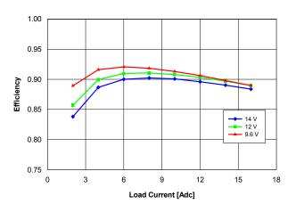
**Fig. 2.0V.2:** Efficiency vs. load current and input voltage for Vout = 2.0 V converter mounted vertically with air flowing at a rate of 200 LFM (1 m/s) and Ta =  $25 \, ^{\circ}\text{C}$ .
