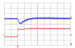
Fig. 1.0V.6: Output voltage response for Vout = 1.0 V to positive load current step change from 8 A to 16 A with slew rate of 5 A/µs at Vin = 12 V. Top trace: output voltage (200 mV/div.); Bottom trace: load current (5 A/div.). Co = 100  $\mu$ F ceramic. Time scale: 20 µs/div.
