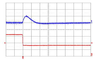
Fig. 1.2V.7: Output voltage response for Vout = 1.2 V to negative load current step change from 16 A to 8 A with slew rate of -5 A/µs at Vin = 12 V. Top trace: output voltage (200 mV/div.); Bottom trace: load current (5 A/div.). Co = 100  $\mu$ F ceramic. Time scale: 20 μs/div.
