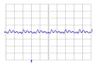
Fig. 0.7525V.5: Output voltage ripple (20 mV/div.) at full rated load current into a resistive load with external capacitance 100 μF ceramic + 1 μF ceramic and Vin = 12 V for Vout = 0.7525 V. Time scale: 2  $\mu$ s/div.
