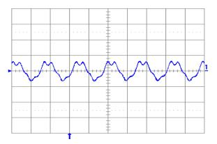
Fig. 5.0V.5: Output voltage ripple (20 mV/div.) at full rated load current into a resistive load with external capacitance 100 μF ceramic + 1 μF ceramic and Vin = 12 V for Vout = 5.0 V. Time scale: 2 µs/div.
