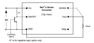
Fig. A: Circuit configuration for ON/OFF function.
