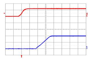
Fig. 2.0V.4: Turn-on transient for Vout = 2.0 V with application of Vin at full rated load current (resistive) and 100 µF external capacitance at Vin = 12 V. Top trace: Vin (10 V/div.); Bottom trace: output voltage (1 V/div.); Time scale: 2 ms/div.
