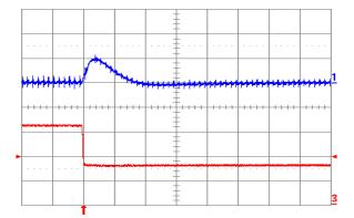
Fig. 1.5V.7: Output voltage response for Vout = 1.5 V to negative load current step change from 16 A to 8 A with slew rate of -5 A/µs at Vin = 12 V. Top trace: output voltage (200 mV/div.); Bottom trace: load current (5 A/div.). Co = 100  $\mu$ F ceramic. Time scale: 20 μs/div.
