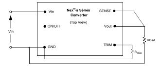
Fig. C: Configuration for programming output voltage.
