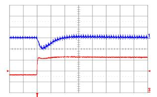
**Fig. 1.8V.6:** Output voltage response for Vout = 1.8 V to positive load current step change from 8 A to 16 A with slew rate of 5 A/ $\mu$ s at Vin = 12 V. Top trace: output voltage (200 mV/div.); Bottom trace: load current (5 A/div.). Co = 100  $\mu$ F ceramic. Time scale: 20  $\mu$ s/div.
