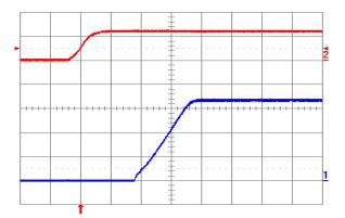
Fig. 3.3V.4: Turn-on transient for Vout = 3.3 V with application of Vin at full rated load current (resistive) and 100 µF external capacitance at Vin = 12 V. Top trace: Vin (10 V/div.); Bottom trace: output voltage (1 V/div.); Time scale: 2 ms/div.
