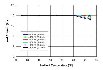
**Fig. 1.0V.1:** Available load current vs. ambient temperature and airflow rates for Vout = 1.0 V converter mounted vertically with Vin = 12 V, and maximum MOSFET temperature  $\leq 120 \, ^{\circ}\text{C}$ .
