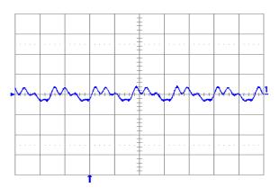
Fig. 2.0V.5: Output voltage ripple (20 mV/div.) at full rated load current into a resistive load with external capacitance 100 μF ceramic + 1 μF ceramic and Vin = 12 V for Vout = 2.0 V. Time scale: 2 µs/div.
