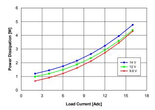
Fig. 5.0V.3: Power Loss vs. load current and input voltage for Vout = 5.0 V converter mounted vertically with air flowing at a rate of 200 LFM (1 m/s) and Ta =  $25 \,^{\circ}\text{C}$ .
