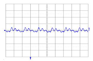
Fig. 1.5V.5: Output voltage ripple (20 mV/div.) at full rated load current into a resistive load with external capacitance 100 μF ceramic + 1 μF ceramic and Vin = 12 V for Vout = 1.5 V. Time scale: 2 μs/div.
