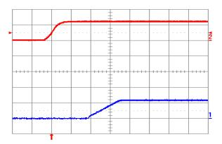
Fig. 1.2V.4: Turn-on transient for Vout = 1.2 V with application of Vin at full rated load current (resistive) and 100 µF external capacitance at Vin = 12 V. Top trace: Vin (10 V/div.); Bottom trace: output voltage (1 V/div.); Time scale: 2 ms/div.
