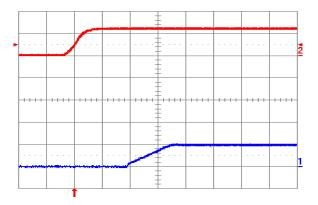
Fig. 1.0V.4: Turn-on transient for Vout = 1.0 V with application of Vin at full rated load current (resistive) and 100 µF external capacitance at Vin = 12 V. Top trace: Vin (10 V/div.); Bottom trace: output voltage (1 V/div.); Time scale: 2 ms/div.
