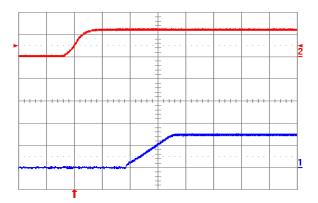
Fig. 1.5V.4: Turn-on transient for Vout = 1.5 V with application of Vin at full rated load current (resistive) and 100 µF external capacitance at Vin = 12 V. Top trace: Vin (10 V/div.); Bottom trace: output voltage (1 V/div.); Time scale: 2 ms/div.
