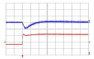
Fig. 0.7525V.6: Output voltage response for Vout = 0.7525 V to positive load current step change from 8 A to 16 A with slew rate of 5 A/µs at Vin = 12 V. Top trace: output voltage (200 mV/div.); Bottom trace: load current (5 A/div.). Co = 100  $\mu$ F ceramic. Time scale: 20 µs/div.
