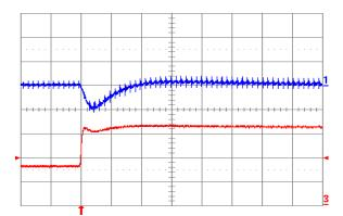
Fig. 1.2V.6: Output voltage response for Vout = 1.2 V to positive load current step change from 8 A to 16 A with slew rate of 5 A/µs at Vin = 12 V. Top trace: output voltage (200 mV/div.); Bottom trace: load current (5 A/div.). Co = 100  $\mu$ F ceramic. Time scale: 20 µs/div.
