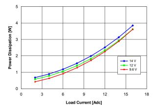
Fig. 1.0V.3: Power loss vs. load current and input voltage for Vout = 1.0 V converter mounted vertically with air flowing at a rate of 200 LFM (1 m/s) and Ta =  $25 \, ^{\circ}\text{C}$ .
