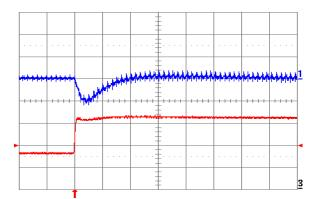
Fig. 2.0V.6: Output voltage response for Vout = 2.0 V to positive load current step change from 8 A to 16 A with slew rate of 5 A/µs at Vin = 12 V. Top trace: output voltage (200 mV/div.); Bottom trace: load current (5 A/div.). Co = 100  $\mu$ F ceramic. Time scale: 20 µs/div.
