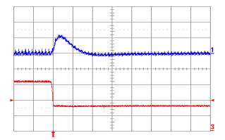
Fig. 3.3V.7: Output voltage response for Vout = 3.3 V to negative load current step change from 16 A to 8 A with slew rate of -5 A/µs at Vin = 12 V. Top trace: output voltage (200 mV/div.); Bottom trace: load current (5 A/div.). Co = 100  $\mu$ F ceramic. Time scale: 20 µs/div.
