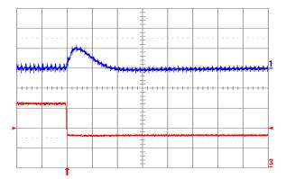
Fig. 2.0V.7: Output voltage response for Vout = 2.0 V to negative load current step change from 16 A to 8 A with slew rate of -5 A/µs at Vin = 12 V. Top trace: output voltage (200 mV/div.); Bottom trace: load current (5 A/div.). Co = 100  $\mu$ F ceramic. Time scale: 20 µs/div.
