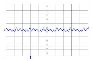
Fig. 1.2V.5: Output voltage ripple (20 mV/div.) at full rated load current into a resistive load with external capacitance 100 μF ceramic + 1 μF ceramic and Vin = 12 V for Vout = 1.2 V. Time scale: 2 μs/div.
