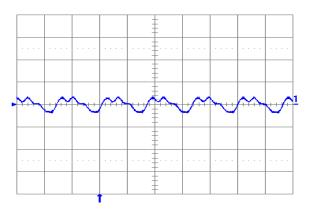
Fig. 2.5V.5: Output voltage ripple (20 mV/div.) at full rated load current into a resistive load with external capacitance 100 μF ceramic + 1 μF ceramic and Vin = 12 V for Vout = 2.5V. Time scale:  $2 \mu s/div$ .
