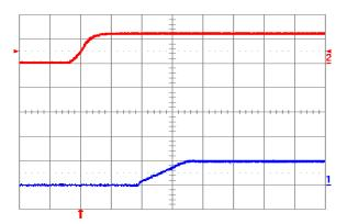
Fig. 0.7525V.4: Turn-on transient for Vout = 0.7525V with application of Vin at full rated load current (resistive) and 100 µF external capacitance at Vin = 12 V. Top trace: Vin (10 V/div.); Bottom trace: output voltage (1 V/div.); Time scale: 2 ms/div.
