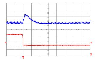
Fig. 5.0V.7: Output voltage response for Vout = 5.0 V to negative load current step change from 16 A to 8 A with slew rate of -5 A/µs at Vin = 12 V. Top trace: output voltage (200 mV/div.); Bottom trace: load current (5A/div.). Co = 100  $\mu$ F ceramic. Time scale: 20 µs/div.
