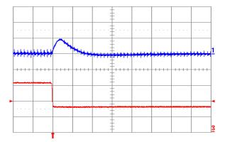
Fig. 1.0V.7: Output voltage response for Vout = 1.0 V to negative load current step change from 16 A to 8 A with slew rate of -5 A/µs at Vin = 12 V. Top trace: output voltage (200 mV/div.); Bottom trace: load current (5 A/div.). Co = 100  $\mu$ F ceramic. Time scale: 20 μs/div.
