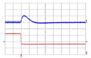
Fig. 2.5V.7: Output voltage response for Vout = 2.5 V to negative load current step change from 16 A to 8 A with slew rate of -5 A/µs at Vin = 12 V. Top trace: output voltage (200 mV/div.); Bottom trace: load current (5 A/div.). Co = 100  $\mu$ F ceramic. Time scale: 20 μs/div.
