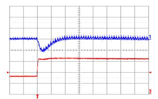
Fig. 3.3V.6: Output voltage response for Vout = 3.3 V to positive load current step change from 8 A to 16 A with slew rate of 5 A/µs at Vin = 12 V. Top trace: output voltage (200 mV/div.); Bottom trace: load current (5 A/div.). Co = 100  $\mu$ F ceramic. Time scale: 20 µs/div.
