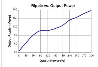
$\begin{array}{l} \textit{Figure 9} & - \textit{Output voltage ripple vs. output power at 48 $V_{IN}$} \\ & \textit{without any external bypass capacitor.} \end{array}$
