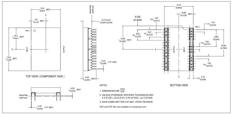
Figure 17 — BCM™ through-hole module mechanical outline
