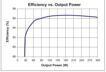
Figure 5 — Efficiency vs. output power
