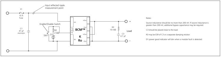
Figure 20 — BCM™ module test circuit
