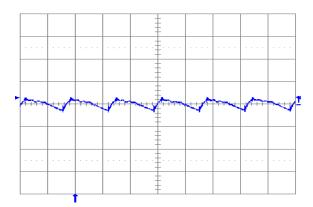
**Fig. 1.8V.6:** Output voltage ripple (20 mV/div.) at full rated load current into a resistive load with external capacitance 100  $\mu$ F ceramic + 1  $\mu$ F ceramic, and Vin = 12 V for Vout = 1.8 V. Time scale: 2  $\mu$ s/div.
