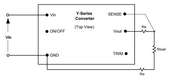
Fig. B: Circuit configuration for ON/OFF function.
