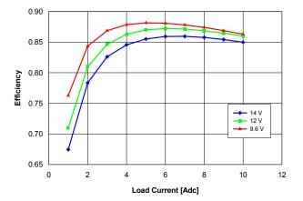
Fig. 1.0V.3: Efficiency vs. load current and input voltage for Vout = 1.0 V converter mounted vertically with air flowing at a rate of 200 LFM (1 m/s) and Ta =  $25 \, ^{\circ}\text{C}$ .
