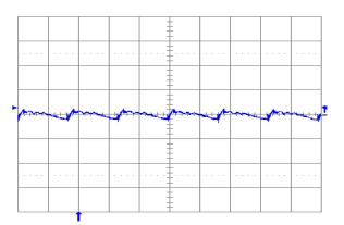
Fig. 1.2V.6: Output voltage ripple (20 mV/div.) at full rated load current into a resistive load with external capacitance 100 µF ceramic + 1  $\mu$ F ceramic, and Vin = 12 V for Vout = 1.2 V. Time scale: 2 µs/div.
