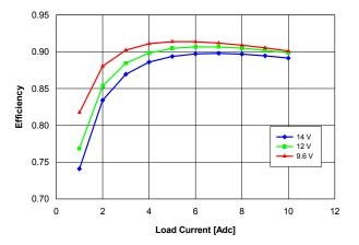
Fig. 1.5V.3: Efficiency vs. load current and input voltage for Vout = 1.5 V converter mounted vertically with air flowing at a rate of 200 LFM (1 m/s) and Ta = 25  $^{\circ}$ C.
