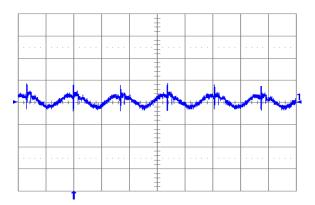
**Fig. 0.7525V.6:** Output voltage ripple (20 mV/div.) at full rated load current into a resistive load with external capacitance 100  $\mu$ F ceramic + 1  $\mu$ F ceramic, and Vin = 12 V for Vout = 0.7525 V. Time scale: 2  $\mu$ s/div.
