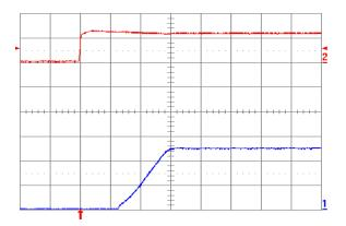
Fig. 2.5V.5: Turn-on transient for Vout = 2.5 V with application of Vin at full rated load current (resistive) and 47 µF external capacitance at Vin = 12 V. Top trace: Vin (10 V/div.); Bottom trace: output voltage (1 V/div.); Time scale: 2 ms/div.
