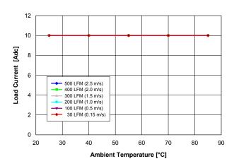
Fig. 3.3V.2: Available load current vs. ambient temperature and airflow rates for Vout = 3.3 V converter mounted horizontally with Vin = 12 V, and maximum MOSFET temperature  $\leq 110$  °C.
