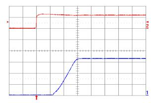
Fig. 3.3V.5: Turn-on transient for Vout = 3.3 V with application of Vin at full rated load current (resistive) and  $100 \mu\text{F}$  external capacitance at Vin = 12 V. Top trace: Vin (10 V/div.); Bottom trace: output voltage (1 V/div.); Time scale: 2 ms/div.
