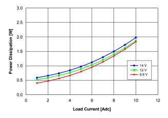
Fig. 2.0V.4: Power loss vs. load current and input voltage for Vout = 2.0 V converter mounted vertically with air flowing at a rate of 200 LFM (1 m/s) and Ta =  $25 \,^{\circ}\text{C}$ .
