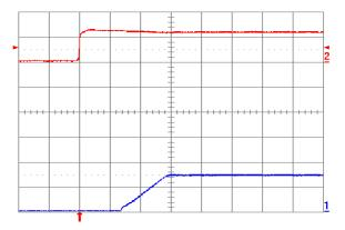
Fig. 1.5V.5: Turn-on transient for Vout = 1.5 V with application of Vin at full rated load current (resistive) and 100  $\mu$ F external capacitance at Vin = 12 V. Top trace: Vin (10 V/div.); Bottom trace: output voltage (1 V/div.); Time scale: 2 ms/div.
