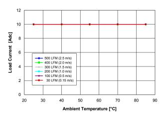
Fig. 1.5V.2: Available load current vs. ambient temperature and airflow rates for Vout = 1.5 V converter mounted horizontally with Vin = 12 V, and maximum MOSFET temperature ≤ 110 °C.
