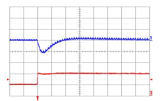
Fig. 1.0V.7: Output voltage response for Vout = 1.0 V to positive load current step change from 5 A to 10 A with slew rate of 5 A/µs at Vin = 12 V. Top trace: output voltage (100 mV/div.); Bottom trace: load current (5 A/div.). Co =100 µF ceramic. Time scale: 20 µs/div.
