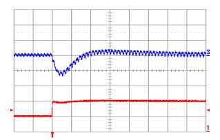
Fig. 2.5V.7: Output voltage response for Vout = 2.5 V to positive load current step change from 5 A to 10 A with slew rate of 5 A/µs at Vin = 12 V. Top trace: output voltage (100 mV/div.); Bottom trace: load current (5 A/div.). Co = 100 µF ceramic. Time scale: 20 µs/div.
