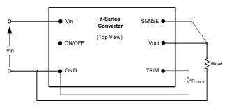
Fig. C: Configuration for programming output voltage.
