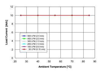
Fig. 2.0V.2: Available load current vs. ambient temperature and airflow rates for Vout = 2.0 V converter mounted horizontally with Vin = 12 V, and maximum MOSFET temperature  $\leq$  110 °C.
