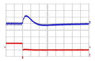
Fig. 2.5V.8: Output voltage response for Vout = 2.5 V to negative load current step change from 10 A to 5 A with slew rate of -5 A/µs at Vin = 12 V. Top trace: output voltage (100 mV/div.); Bottom trace: load current (5 A/div.). Co = 100 µF ceramic. Time scale: 20 µs/div.
