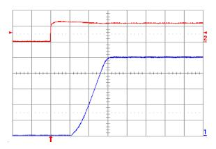
**Fig. 5.0V.5:** Turn-on transient for Vout = 5.0 V with application of Vin at full rated load current (resistive) and  $100 \mu\text{F}$  external capacitance at Vin = 12 V. Top trace: Vin (10 V/div.); Bottom trace: output voltage (1 V/div.); Time scale: 2 ms/div.
