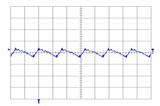
Fig. 2.5V.6: Output voltage ripple (20 mV/div.) at full rated load current into a resistive load with external capacitance 100  $\mu F$  ceramic + 1  $\mu F$  ceramic, and Vin = 12 V for Vout = 2.5 V. Time scale: 2 µs/div.
