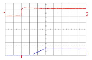
Fig. 1.0V.5: Turn-on transient for Vout = 1.0 V with application of Vin at full rated load current (resistive) and 100 µF external capacitance at Vin = 12 V. Top trace: Vin (10 V/div.); Bottom trace: output voltage (1 V/div.); Time scale: 2 ms/div.
