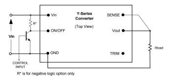
Fig. A: Circuit configuration for ON/OFF function.
