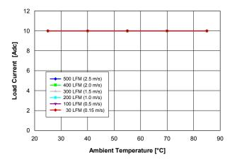
Fig. 1.2V.1: Available load current vs. ambient temperature and airflow rates for Vout = 1.2 V converter mounted vertically with Vin = 12 V, and maximum MOSFET temperature ≤ 110 °C.
