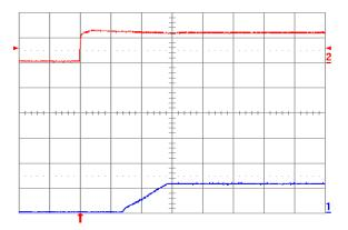
Fig. 1.2V.5: Turn-on transient for Vout = 1.2 V with application of Vin at full rated load current (resistive) and 100 µF external capacitance at Vin = 12 V. Top trace: Vin (10 V/div.); Bottom trace: output voltage (1 V/div.); Time scale: 5 ms/div.
