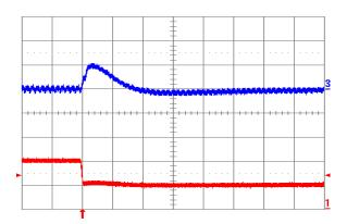
Fig. 1.2V.8: Output voltage response for Vout = 1.2 V to negative load current step change from 10 A to 5 A with slew rate of -5 A/µs at Vin = 12 V. Top trace: output voltage (100 mV/div.); Bottom trace: load current (5 A/div.). Co = 100 µF ceramic. Time scale: 20 µs/div.
