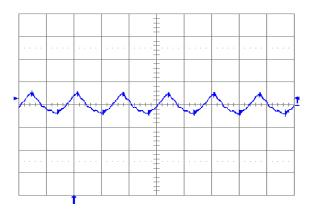
**Fig. 5.0V.6:** Output voltage ripple (20 mV/div.) at full rated load current into a resistive load with external capacitance 100  $\mu$ F ceramic + 1  $\mu$ F ceramic, and Vin = 12 V for Vout = 5.0 V. Time scale: 2  $\mu$ s/div.
