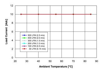
Fig. 3.3V.1: Available load current vs. ambient temperature and airflow rates for Vout = 3.3 V converter mounted vertically with Vin = 12 V, and maximum MOSFET temperature  $\leq$  110 °C.
