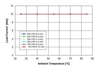
Fig. 1.8V.2: Available load current vs. ambient temperature and airflow rates for Vout = 1.8 V converter mounted horizontally with Vin = 12 V, and maximum MOSFET temperature ≤ 110 °C.
