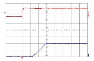
Fig. 2.0V.5: Turn-on transient for Vout = 2.0 V with application of Vin at full rated load current (resistive) and  $100 \mu\text{F}$  external capacitance at Vin = 12 V. Top trace: Vin (10 V/div.); Bottom trace: output voltage (1 V/div.); Time scale: 2 ms/div.
