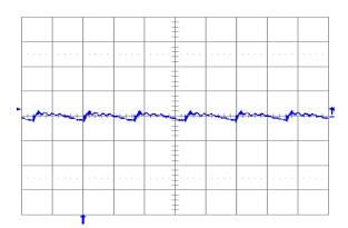
Fig. 1.0V.6: Output voltage ripple (20 mV/div.) at full rated load current into a resistive load with external capacitance 100 µF ceramic + 1  $\mu$ F ceramic, and Vin = 12 V for Vout = 1.0 V. Time scale: 2 µs/div.
