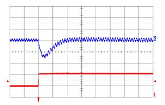
**Fig. 5.0V.7:** Output voltage response for Vout = 5.0 V to positive load current step change from 5 A to 10 A with slew rate of 5 A/µs at Vin = 12 V. Top trace: output voltage (100 mV/div.); Bottom trace: load current (5 A/div.). Co = 100 µF ceramic. Time scale: 20 µs/div.
