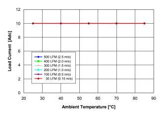
Fig. 2.0V.1: Available load current vs. ambient temperature and airflow rates for Vout = 2.0 V converter mounted vertically with Vin = 12 V, and maximum MOSFET temperature  $\leq 110 \text{ °C}$ .
