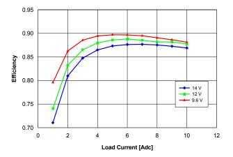
Fig. 1.2V.3: Efficiency vs. load current and input voltage for Vout = 1.2 V converter mounted vertically with air flowing at a rate of 200 LFM (1 m/s) and Ta = 25  $^{\circ}$ C.
