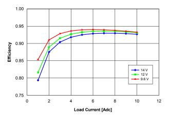
Fig. 2.5V.3: Efficiency vs. load current and input voltage for Vout = 2.5 V converter mounted vertically with air flowing at a rate of 200 LFM (1 m/s) and Ta = 25  $^{\circ}$ C.
