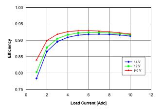
Fig. 2.0V.3: Efficiency vs. load current and input voltage for Vout = 2.0 V converter mounted vertically with air flowing at a rate of 200 LFM (1 m/s) and Ta =  $25 \, ^{\circ}\text{C}$ .
