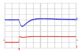
Fig. 1.2V.7: Output voltage response for Vout = 1.2 V to positive load current step change from 5 A to 10 A with slew rate of 5 A/µs at Vin = 12 V. Top trace: output voltage (100 mV/div.); Bottom trace: load current (5 A/div.). Co = 100 µF ceramic. Time scale: 20 µs/div.
