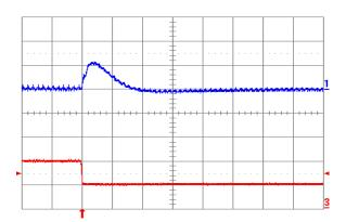
Fig. 1.0V.8: Output voltage response for Vout = 1.0 V to negative load current step change from 10 A to 5 A with slew rate of -5 A/µs at Vin = 12 V. Top trace: output voltage (100 mV/div.); Bottom trace: load current (5 A/div.). Co = 100 µF ceramic. Time scale: 20 µs/div.
