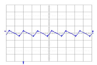
**Fig. 3.3V.6:** Output voltage ripple (20 mV/div.) at full rated load current into a resistive load with external capacitance 100  $\mu$ F ceramic + 1  $\mu$ F ceramic, and Vin = 12 V for Vout = 3.3 V. Time scale: 2  $\mu$ s/div.
