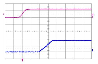
**Fig. 0.7525 V.5**: Turn-on transient for Vout = 0.7525 V with application of Vin at full rated load current (resistive) and 100  $\mu$ F external capacitance at Vin = 12 V. Top trace: Vin (10 V/div.); Bottom trace: output voltage (0.5 V/div.); Time scale: 2 ms/div
