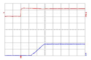
Fig. 1.8V.5: Turn-on transient for Vout = 1.8 V with application of Vin at full rated load current (resistive) and 100  $\mu$ F external capacitance at Vin = 12 V. Top trace: Vin (10 V/div.); Bottom trace: output voltage (1 V/div.); Time scale: 2 ms/div.
