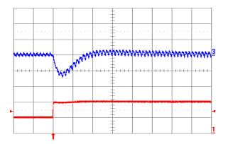
Fig. 3.3V.7: Output voltage response for Vout = 3.3 V to positive load current step change from 5 A to 10 A with slew rate of 5 A/ $\mu$ s at Vin = 12 V. Top trace: output voltage (100 mV/div.); Bottom trace: load current (5 A/div.). Co =  $100 \text{ }\mu\text{F}$  ceramic. Time scale: 20 us/div.
