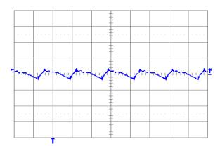
**Fig. 2.0V.6:** Output voltage ripple (20 mV/div.) at full rated load current into a resistive load with external capacitance 100  $\mu$ F ceramic + 1  $\mu$ F ceramic, and Vin = 12 V for Vout = 2.0 V. Time scale: 2  $\mu$ s/div.
