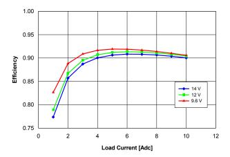
Fig. 1.8V.3: Efficiency vs. load current and input voltage for Vout = 1.8 V converter mounted vertically with air flowing at a rate of 200 LFM (1 m/s) and Ta = 25  $^{\circ}$ C.
