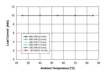
Fig. 0.7525V.2: Available load current vs. ambient temperature and airflow rates for Vout = 0.7525 V converter mounted horizontally with Vin = 12 V, and maximum MOSFET temperature  $\leq$  110 °C.
