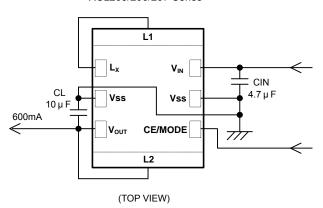
\* "L1 and Lx", and "L2 and Vout" is connected by wiring.
