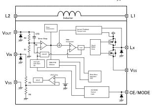
NOTE: The XCL205 offers a fixed PWM control, a signal from CE/MODE Control Logic to PWM/PFM Selector is fixed to "L" level inside. The XCL206 control scheme is PWM/PFM automatic switching, a signal from CE/MODE Control Logic to PWM/PFM Selector is fixed to "H" level inside. The diodes placed inside are ESD protection diodes and parasitic diodes.
