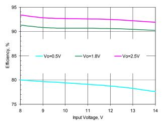
Figure 5. Efficiency vs. Input Voltage. Iout=60A
