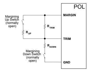
Figure 13. Alternative Margining Configuration
