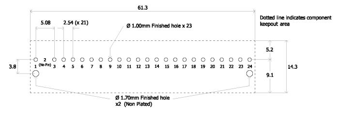
Figure 15. Recommended Footprint - Top View
