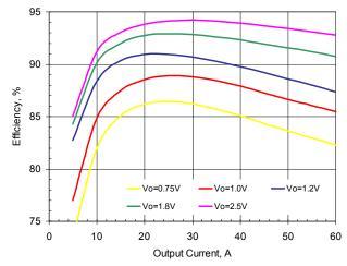
Figure 3. Efficiency vs. Load. Vin=12V
