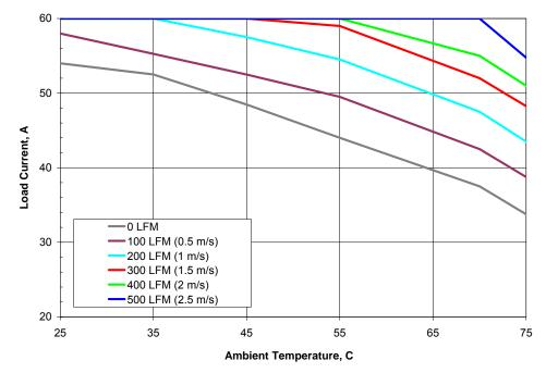
Figure 10. Thermal Derating Curves. Vin=12V, Vout=2.5V
