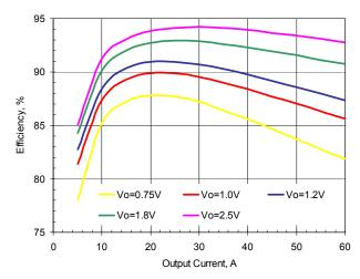
Figure 2. Efficiency vs. Load. Vin=9.6V
