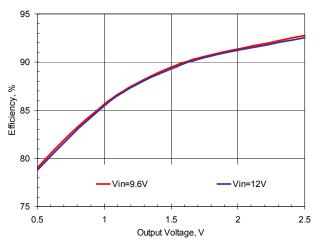
Figure 4. Efficiency vs. Output Voltage, lout=60A
