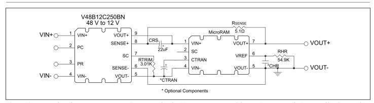
Figure 10 — Typical configuration using Remote Sense control and a 12 V converter trimmed down to 9 V. R<sub>HR</sub> set for 375 mV of headroom voltage
