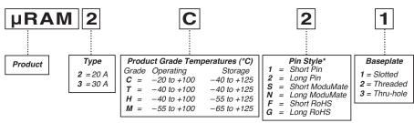
\*Pin styles S & N are compatible with the ModuMate interconnect system for socketing and surface mounting.
