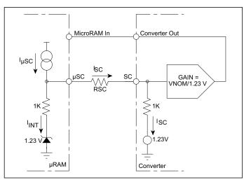
Figure 9 — MicroRAM's SC control circuit.
