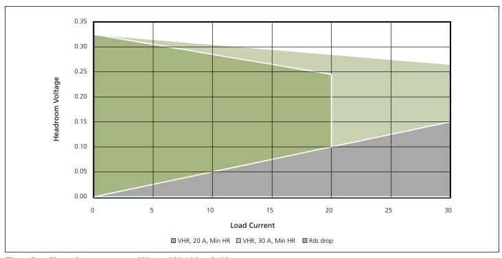
Figure 5 — Slope adjust comparison of 20 A and 30 A MicroRAM.
