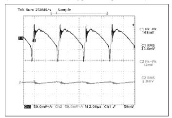
Figure 22 — V375B12C250B and µRAM; Input and output ripple@50% (10 A) load CH1=Vi; CH2=Vo; Vi-Vo=305 mV; RHR=80 k (Configured as in Figure 7 w/o Trim)
