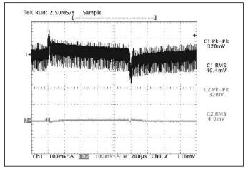
Figure 23 — V300B12C250B and µRAM; Input and output dynamic response no added CTRAN; 17.5% of 20 A rating load step of 3.5 A (10 A – 13.5 A);RHR=80 k (Configured as in Figure 7 w/o Trim)
