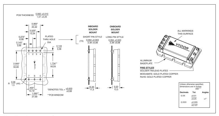
Figure 29 — PCB mounting specifications
