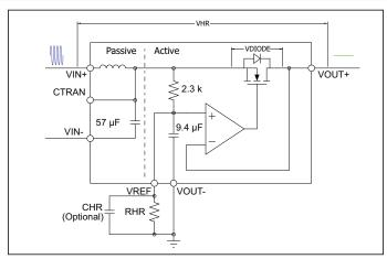
Figure 1 — Simplified MicroRAM Block Diagram
