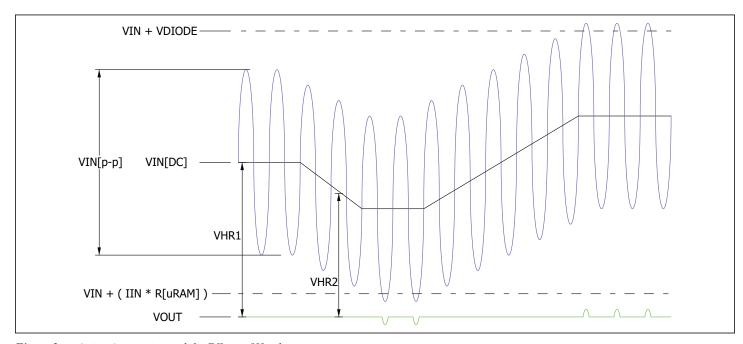
Figure 3 — Active Attenuation and the Effects of Headroom
