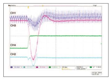
Figure 6 — Normal transient load response
