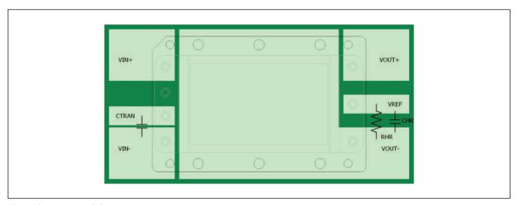
Figure 18 — Recommended copper patterns, top view.
