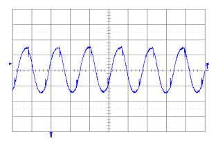
Fig. 2.0V.6: Output voltage ripple (20 mV/div.) at full rated load current into a resistive load with external capacitance 10  $\mu F$  ceramic + 1  $\mu F$  ceramic and Vin = 5 V for Vout = 2.0 V. Time scale:  $2 \mu \text{s/div}$ .
