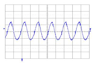
**Fig. 1.5V.6:** Output voltage ripple (20 mV/div.) at full rated load current into a resistive load with external capacitance 10  $\mu$ F ceramic + 1  $\mu$ F ceramic and Vin = 5 V for Vout = 1.5 V. Time scale: 2  $\mu$ s/div.
