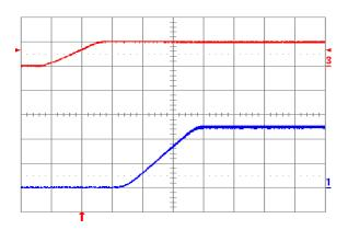
**Fig. 2.5V.4:** Turn-on transient for Vout = 2.5 V with application of Vin at full rated load current (resistive) and 47 μF external capacitance at Vin = 5 V. Top trace: Vin (5 V/div.); Bottom trace: output voltage (1V/div.); Time scale: 2 ms/div.
