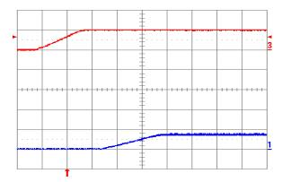
**Fig. 0.7525V.4:** Turn-on transient for Vout = 0.7525 V with application of Vin at full rated load current (resistive) and 47 μF external capacitance at Vin = 5 V. Top trace: Vin (5 V/div.); Bottom trace: output voltage (1 V/div.); Time scale: 2 ms/div.
