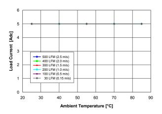
Fig. 1.2V.2: Available load current vs. ambient temperature and airflow rates for Vout = 1.2 V converter mounted horizontally with Vin = 5 V, air flowing from pin 5 to pin 1 and maximum MOSFET temperature ≤ 120 °C.
