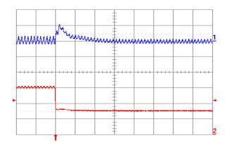
Fig. 1.2V.8: Output voltage response for Vout = 1.2 V to negative load current step change from 5 A to 2.5 A with slew rate of -5 A/µs at Vin = 5 V. Top trace: output voltage (100 mV/div.); Bottom trace: load current (2 A/div.). Co = 47 μF ceramic + 1 μF ceramic. Time scale: 20 μs/div.
