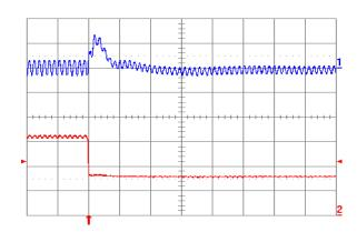
**Fig. 2.5V.8:** Output voltage response for Vout = 2.5 V to negative load current step change from 5 A to 2.5 A with slew rate of -5 A/µs at Vin = 5 V. Top trace: output voltage (100 mV/div.); Bottom trace: load current (2 A/div.). Co = 47 µF ceramic + 1 µF ceramic. Time scale: 20 µs/div.
