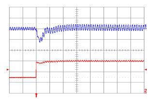
Fig. 1.8V.7: Output voltage response for Vout = 1. 8V to positive load current step change from 2.5 A to 5 A with slew rate of 5 A/µs at Vin = 5 V. Top trace: output voltage (100 mV/div.); Bottom trace: load current (2 A/div.). Co = 47 μF ceramic + 1 μF ceramic. Time scale: 20 μs/div.
