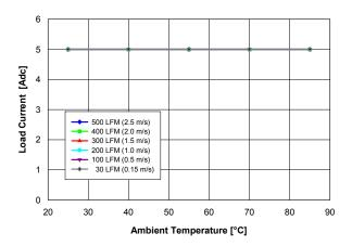
Fig. 1.0V.1: Available load current vs. temperature and airflow rates for Vout = 1.0 V converter mounted vertically with Vin = 5 V, air flowing from pin 5 to pin 1 and maximum MOSFET temperature ≤ 120 °C.
