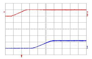
Fig. 1.2V.5: Turn-on transient for Vout = 1.2 V with application of Vin at full rated load current (resistive) and 47 μF external capacitance at Vin = 5 V. Top trace: Vin (5 V/div.); Bottom trace: output voltage (1 V/div.); Time scale: 2 ms/div.
