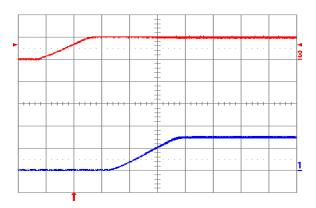
**Fig. 1.5V.5:** Turn-on transient for Vout = 1.5 V with application of Vin at full rated load current (resistive) and  $47 \mu F$  external capacitance at Vin = 5 V. Top trace: Vin (5 V/div.); Bottom trace: output voltage (1 V/div.); Time scale: 2 ms/div.
