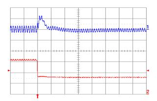
Fig. 2.0V.8: Output voltage response for Vout = 2.0 V to negative load current step change from 5 A to 2.5 A with slew rate of -5 A/µs at Vin = 5 V. Top trace: output voltage (100 mV/div.); Bottom trace: load current (2 A/div.). Co = 47 μF ceramic + 1 μF ceramic. Time scale: 20 μs/div.
