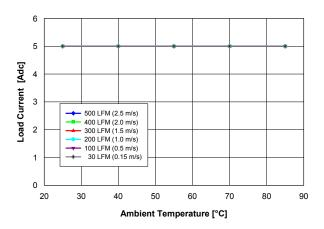
**Fig. 2.0V.1:** Available load current vs. ambient temperature and airflow rates for Vout = 2.0 V converter mounted vertically with Vin = 5 V, air flowing from pin 5 to pin 1 and maximum MOSFET temperature  $\leq 120 \text{ °C}$ .
