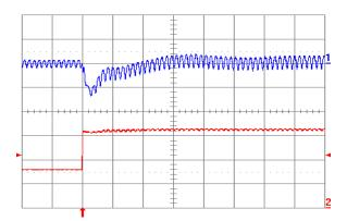
**Fig. 3.3V.7:** Output voltage response for Vout = 3.3 V to positive load current step change from 2.5 A to 5 A with slew rate of  $5 \text{ A/}\mu\text{s}$  at Vin = 5 V. Top trace: output voltage (100 mV/div.); Bottom trace: load current (2 A/div.). Co =  $47 \mu\text{F}$  ceramic +  $1 \mu\text{F}$  ceramic. Time scale:  $20 \mu\text{s/div.}$
