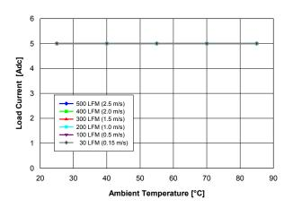
Fig. 1.0V.2: Available load current vs. ambient temperature and airflow rates for Vout = 1.0 V converter mounted horizontally with Vin = 5 V, air flowing from pin 5 to pin 1 and maximum MOSFET temperature ≤ 120 °C.
