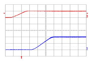
Fig. 2.0V.5: Turn-on transient for Vout = 2.0 V with application of Vin at full rated load current (resistive) and 47 µF external capacitance at Vin = 5 V. Top trace: Vin (5 V/div.); Bottom trace: output voltage (1 V/div.); Time scale: 2 ms/div.
