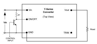
Fig. A: Circuit configuration for ON/OFF function.
