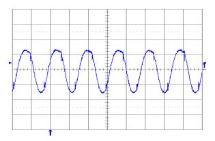
**Fig. 2.5V.5:** Output voltage ripple (20 mV/div.) at full rated load current into a resistive load with external capacitance 10  $\mu$ F ceramic + 1  $\mu$ F ceramic and Vin = 5 V for Vout = 2.5 V. Time scale: 2  $\mu$ s/div.
