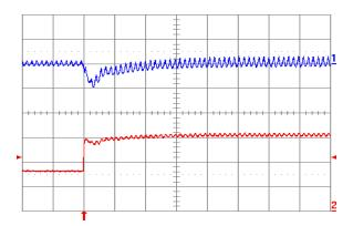
Fig. 0.7525V.7: Output voltage response for Vout = 0.7525 V to positive load current step change from 2.5 A to 5 A with slew rate of 5 A/ $\mu$ s at Vin = 5 V. Top trace: output voltage (100 mV/div.); Bottom trace: load current (2 A/div.). Co = 47  $\mu$ F ceramic + 1  $\mu$ F ceramic. Time scale: 20 µs/div.
