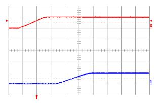
Fig. 1.0V.5: Turn-on transient for Vout = 1.0 V with application of Vin at full rated load current (resistive) and 47 μF external capacitance at Vin = 5 V. Top trace: Vin (5 V/div.); Bottom trace: output voltage (1 V/div.); Time scale: 2 ms/div.
