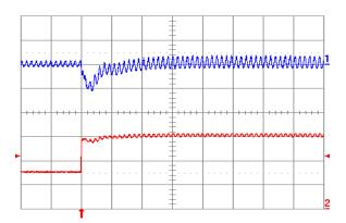
Fig. 1.2V.6: Output voltage response for Vout = 1.2 V to positive load current step change from 2.5 A to 5 A with slew rate of 5 A/µs at Vin = 5 V. Top trace: output voltage (100 mV/div.); Bottom trace: load current (2 A/div.). Co = 47 μF ceramic + 1 μF ceramic. Time scale: 20 μs/div.
