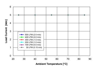
Fig. 1.2V.1: Available load current vs. temperature and airflow rates for Vout = 1.2 V converter mounted vertically with Vin = 5 V, air flowing from pin 5 to pin 1 and maximum MOSFET temperature ≤ 120 °C.
