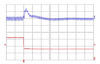
**Fig. 3.3V.8:** Output voltage response for Vout = 3.3 V to negative load current step change from 5 A to 2.5 A with slew rate of -5 A/µs at Vin = 5 V. Top trace: output voltage (100 mV/div.); Bottom trace: load current (2 A/div.). Co = 47 µF ceramic + 1 µF ceramic. Time scale: 20 µs/div.
