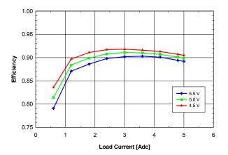
**Fig. 2.0V.3:** Efficiency vs. load current and input voltage for Vout = 2.0 V converter mounted vertically with air flowing from pin 5 to pin 1 at a rate of 200 LFM (1 m/s) and Ta =  $25 \,^{\circ}\text{C}$ .
