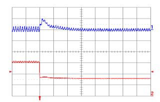
Fig. 1.0V.8: Output voltage response for Vout = 1.0 V to negative load current step change from 5 A to 2.5 A with slew rate of -5 A/µs at Vin = 5 V. Top trace: output voltage (100 mV/div.); Bottom trace: load current (2 A/div.). Co = 47 μF ceramic + 1 μF ceramic. Time scale: 20 μs/div.
