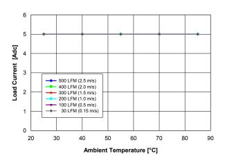
**Fig. 2.0V.2:** Available load current vs. ambient temperature and airflow rates for Vout = 2.0 V converter mounted horizontally with Vin = 5 V, air flowing from pin 5 to pin 1 and maximum MOSFET temperature  $\leq 120 \text{ °C}$ .
