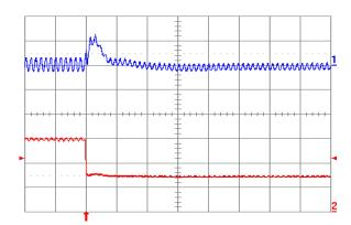
Fig. 1.8V.8: Output voltage response for Vout = 1.8 V to negative load current step change from 5 A to 2.5 A with slew rate of -5 A/µs at Vin = 5 V. Top trace: output voltage (100 mV/div.): Bottom trace: load current (2 A/div.). Co = 47 µF ceramic + 1 µF ceramic. Time scale: 20 µs/div.
