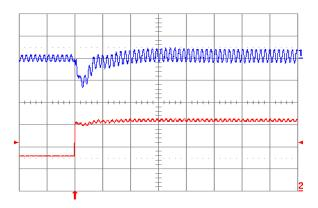
Fig. 2.0V.7: Output voltage response for Vout = 2.0 V to positive load current step change from 2.5 A to 5 A with slew rate of 5 A/µs at Vin = 5 V. Top trace: output voltage (100 mV/div.); Bottom trace: load current (2 A/div.). Co = 47 μF ceramic + 1 μF ceramic. Time scale: 20 μs/div.
