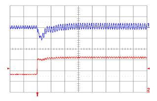
**Fig. 1.5V.7:** Output voltage response for Vout = 1.5 V to positive load current step change from 2.5 A to 5 A with slew rate of 5 A/µs at Vin = 5 V. Top trace: output voltage (100 mV/div.); Bottom trace: load current (2 A/div.). Co = 47 µF ceramic + 1 µF ceramic. Time scale: 20 µs/div.
