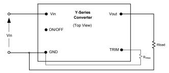
Fig. B: Configuration for programming output voltage.
