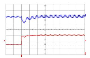
Fig. 1.0V.7: Output voltage response for Vout = 1.0 V to positive load current step change from 2.5 A to 5 A with slew rate of 5 A/µs at Vin = 5 V. Top trace: output voltage (100 mV/div.); Bottom trace: load current (2 A/div.). Co = 47 μF ceramic + 1 μF ceramic. Time scale: 20 μs/div.
