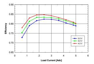
**Fig. 0.7525V.3:** Efficiency vs. load current and input voltage for Vout = 0.7525 V converter mounted vertically with air flowing from pin 5 to pin 1 at a rate of 200 LFM (1 m/s) and Ta = 25 °C.
