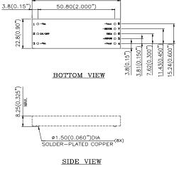
NOTES: DIMENSIONS ARE IN MILLIMETERS AND (INCHES) TOLERANCES: X.Xmm±0.5mm(X.XX in.±0.02 in.) X.XXmm±0.25mm(X.XXX in.±0.010 in.)
