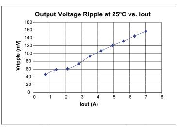
**Figure 7** — Vripple vs. I<sub>OUT</sub>; 384 V<sub>IN</sub>, no external capacitance
