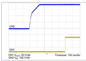
**Figure 9** —  $V_{IN}$  to  $V_{OUT}$  start up waveform
