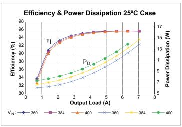
Figure 4 — Efficiency and power dissipation at 25°C (case); V<sub>IN</sub>
