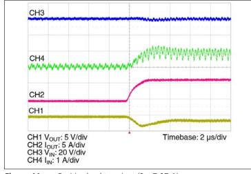
**Figure 11** — Positive load transient (0 – 7.07 A)
