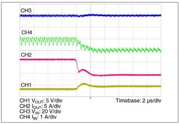
**Figure 12** — Negative load transient (7.07 A – 0 A)
