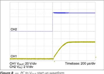
**Figure 8** — PC to  $V_{OUT}$  start up waveform
