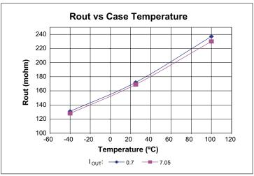
**Figure 6** — R<sub>OUT</sub> vs. temperature vs. I<sub>OUT</sub>
