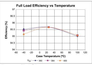
**Figure 2** — Full load efficiency vs. temperature;  $V_{IN}$
