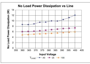
**Figure 1** — No load power dissipation vs.  $V_{IN}$ ;  $T_{CASE}$
