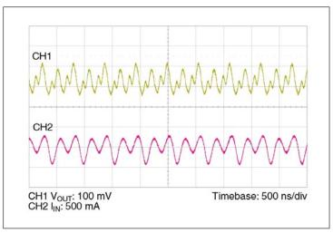
Figure 10 — Output voltage and input current ripple, 384 V<sub>IN</sub>, 325 W no C<sub>OUT</sub>
