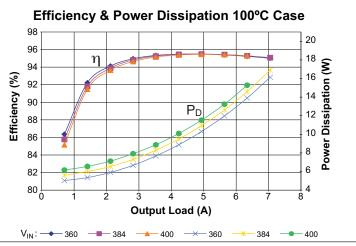
**Figure 5** — Efficiency and power dissipation at 100°C (case); V<sub>IN</sub>
