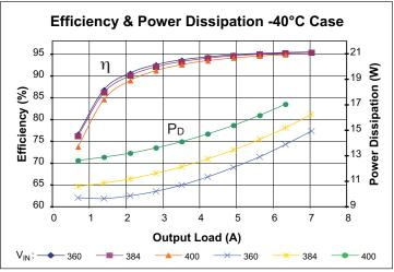
Figure 3 — Efficiency and power dissipation at -40°C (case); V<sub>IN</sub>
