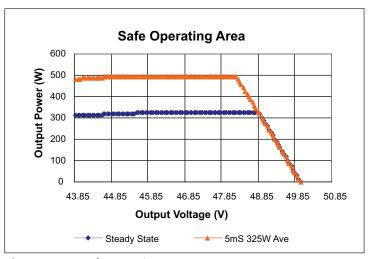
**Figure 14** — Safe Operating Area vs. V<sub>OUT</sub>
