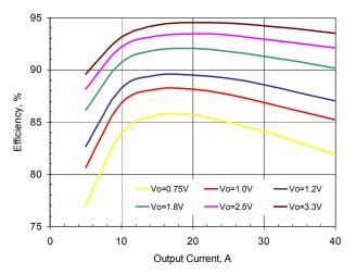
Figure 3. Efficiency vs. Load. Vin=12V
