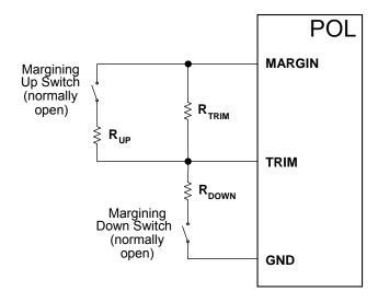
Figure 13. Alternative Margining Configuration
