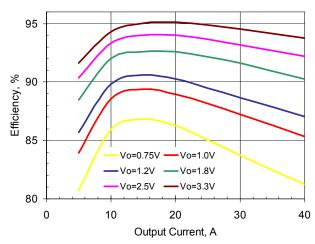
Figure 2. Efficiency vs. Load. Vin=9.6V
