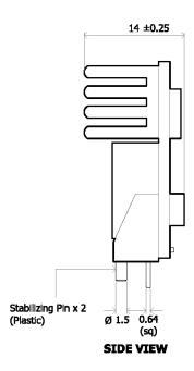
Figure 14. Mechanical Drawing
