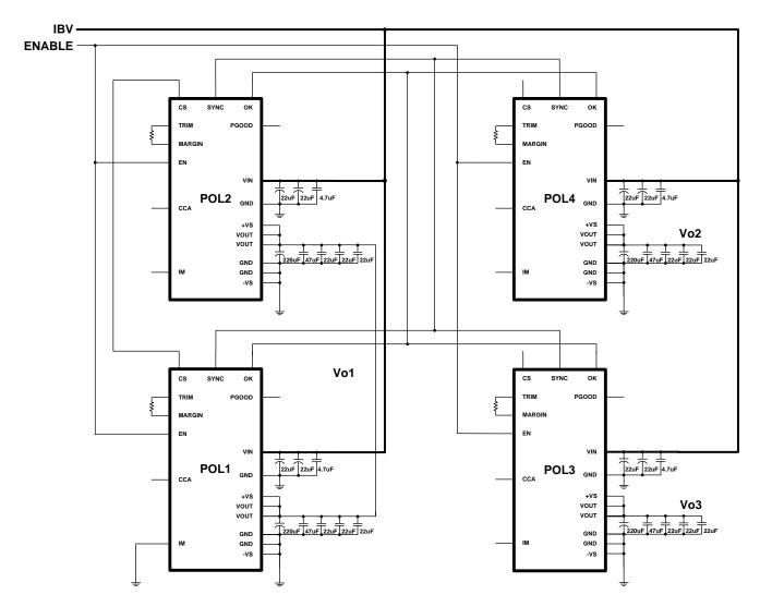
Figure 11. Complete Schematic of Application with Three Independent Outputs. Intermediate Bus Voltage is from 8V to 14V.
