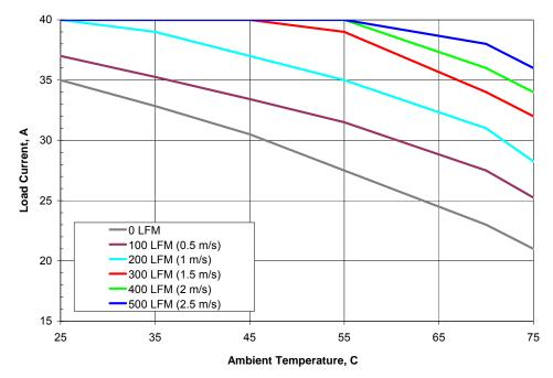
Figure 10. Thermal Derating Curves. Vin=12V, Vout=3.3V
