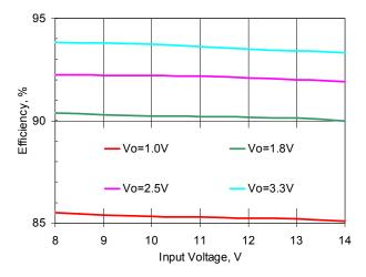
Figure 5. Efficiency vs. Input Voltage. Iout=40A
