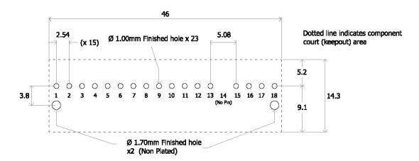
Figure 15. Recommended Footprint - Top View
