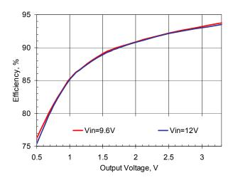
Figure 4. Efficiency vs. Output Voltage, lout=40A
