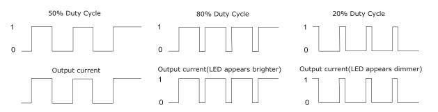
For the rated frequency PWM dimming, the output current of driver matters to the pulse width of the PWM signal, and the numerate please refer to the following formula:
