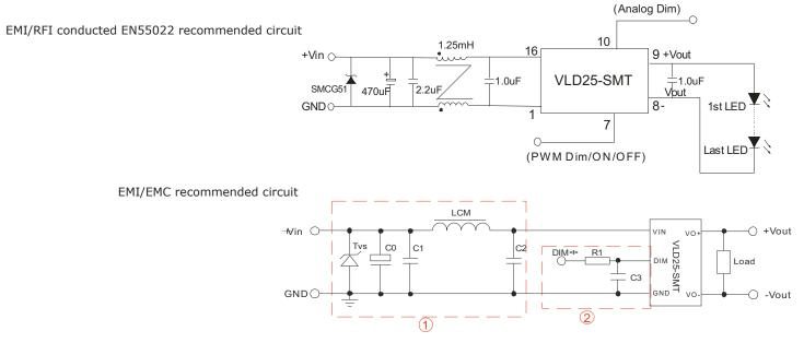
Notes: 1. DIM pin is the module's PWM dimming pin 2. While adding circuit, it may extend the PWM dimming output reaction time
