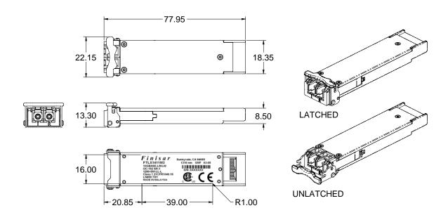
XFP Transceiver (dimensions are in mm)
