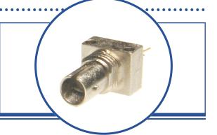
The OPF342 family fiber optic transmitters are high performance devices packaged for data communication links. This transmitter is an 850nm GaAlAs LED and is specifically designed to efficiently launch optical power into fibers ranging in size from 50/125µm up to 200/300µm diameter fiber. Multiple power ranges with upper and lower limits are offered which allows the designer to select a device best suited for the application.
