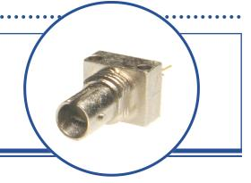
The OPF482 is a low noise silicon PIN photodiode mounted in a low cost package for fiber optic applications. It offers fast response at moderate bias and is compatible with LED and laser diode sources in the 800-1000 nm wavelength region. Low capacitance improves signal to noise performance in typical short haul LAN applications.
