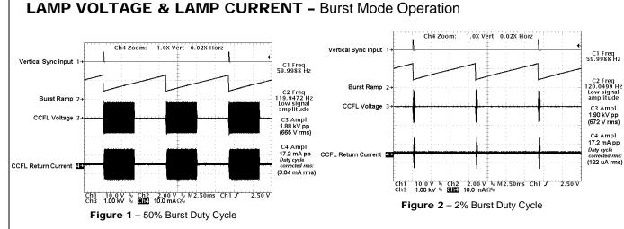
Rather than using the traditional dimming technique of varying lamp current magnitude to adjust light output, RangeMAX inverters use a fixed lamp current value with a duty cycle control method.
