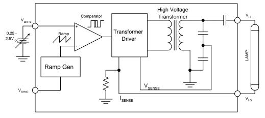
Figure 4 – RangeMAX Block Diagram
