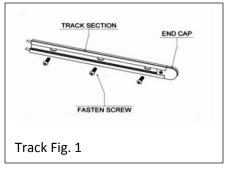
Place the track against your desired mounting location. Tighten fastening screws securely through all mounting holes of track section.
