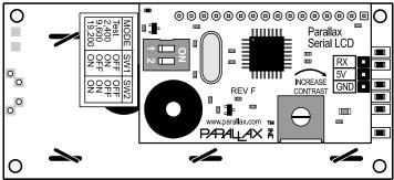
As you can see from the table, there is also a fourth choice called Test. Use this Test mode to confirm that the power and ground to the LCD are hooked up correctly before you send it any data. Move the dip switches to the Test setting and turn on the power. The LCD display should turn on, with the backlight on for models 27977 and 27979, and display the following text:
