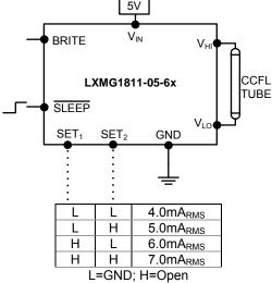
Figure 2 – Max Output Current (SET<sub>1</sub> and SET<sub>2</sub> Inputs)
