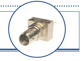
The OPF372 family fiber optic transmitters are high performance devices packaged for data communication links. This transmitter is an 850nm GaAlAs LED and is specifically designed to efficiently launch optical power into fibers ranging in size from 50/125µm up to 200/300µm diameter fiber. Multiple power ranges with upper and lower limits are offered which allows the designer to select a device best suited for the application.
