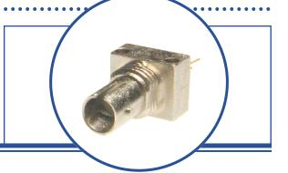
The OPF392 family fiber optic transmitters are high performance devices packaged for data communication links. This transmitter is an 850nm GaAlAs LED and is specifically designed to efficiently launch optical power into fibers ranging in size from 50/125µm up to 200/300µm diameter fiber. Multiple power ranges with upper and lower limits are offered which allows the designer to select a device best suited for the application.
