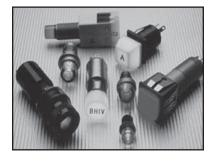
**Material and Finishes** Mounting tube and nut, stainless steel, passivated per MIL-S-5002. Wire leads #26 GA silver coated, stranded copper with TFE-fluro-carbon insulation. Lens Assembly Lens, high impact-resistant plastic per L-P-393 (polycarbonate). Lamp
