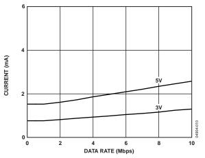
Figure 10. Typical ADuM1310 V<sub>DD2</sub> Supply Current vs. Data Rate for 5 V and 3 V Operation (No Output Load)
