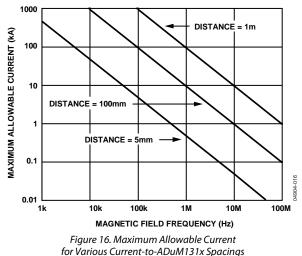
Note that, at combinations of strong magnetic field and high frequency, any loops formed by printed circuit board traces can induce error voltages sufficient to trigger succeeding circuitry. Care should be taken in the layout of such traces to avoid this possibility.
