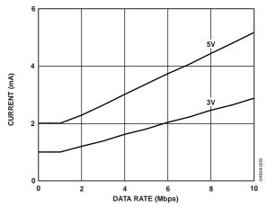
Figure 9. Typical ADuM1310 V<sub>DD1</sub> Supply Current vs. Data Rate for 5 V and 3 V Operation
