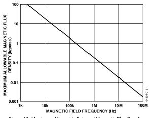
Figure 15. Maximum Allowable External Magnetic Flux Density
