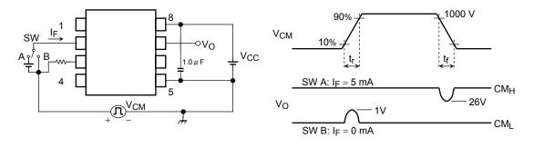
$$CM_{L} = \frac{800(V)}{t_{r}(\mu s)} \qquad CM_{H} = \frac{800(V)}{t_{f}(\mu s)}$$
