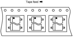
Figure 1 Device Orientation
