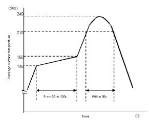
• An example of a temperature profile when lead(Pb)-free solder is used:
