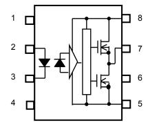
1: N.C 2: Anode 3: Cathode 4: N.C 5: GND 6: N.C 7: VO (output) 8: VCC
