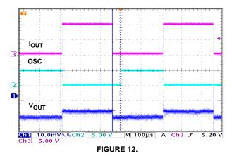
Channel 3 --- sinking and sourcing 5mA current
