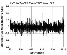
FIGURE 1. DIFFERENTIAL NONLINEARITY vs CODE
