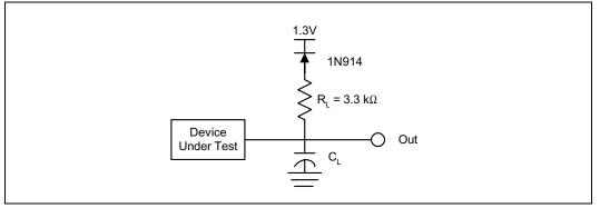
**NOTE:**  $C_L$  Includes Jig Capacitance
