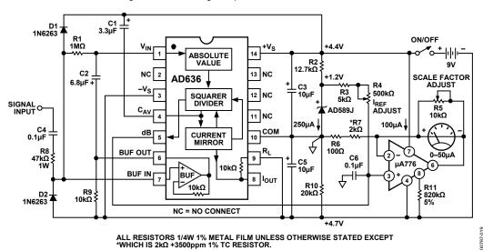
Figure 18. Low Power, High Input Impedance dB Meter
