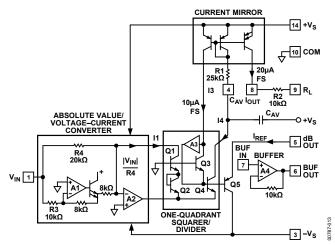
Figure 12. Simplified Schematic
