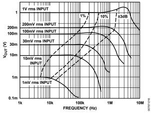
Figure 15. AD636 Frequency Response
