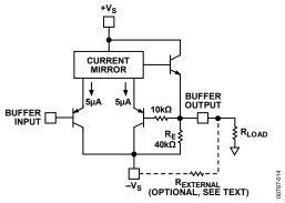
Figure 13. AD636 Buffer Amplifier Simplified Schematic
