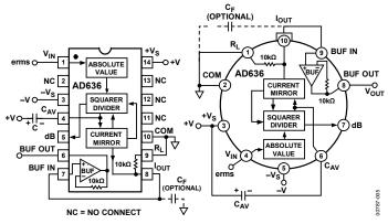
Figure 4. Standard RMS Connection
