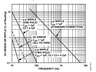
Figure 11. Performance Features of Various Filter Types
