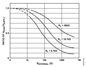
Figure 14. Ratio of Peak Negative Swing to  $-V_s$  vs. R<sub>EXTERNAL</sub> for Several Load Resistances
