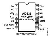
Figure 2. 14-Lead SBDIP Pin Configuration
