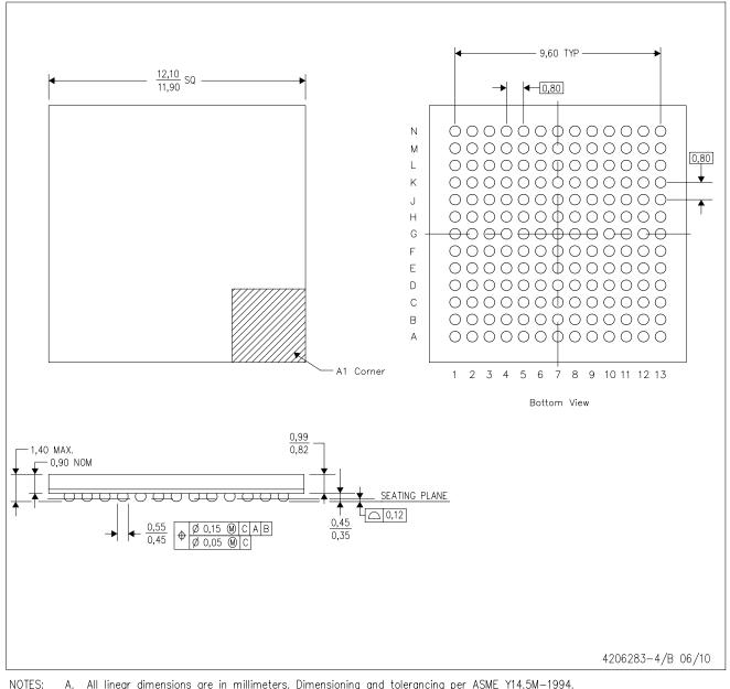
Α. All linear dimensions are in millimeters. Dimensioning and tolerancing per ASME Y14.5M-1994.
