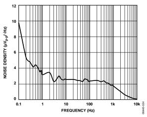
Figure 23. ADR3450 Output Noise Spectral Density
