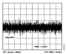
Figure 16. ADR3425 Output Voltage Noise (10 Hz to 10 kHz)
