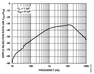
Figure 18. ADR3425 Ripple Rejection Ratio vs. Frequency
