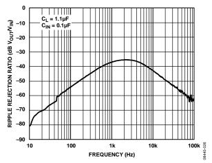
Figure 24. ADR3450 Ripple Rejection Ratio vs. Frequency
