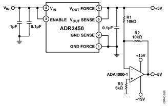
Figure 43. ADR3450 Bipolar Output Reference
