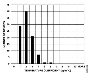
Figure 10. ADR3450 Temperature Coefficient Distribution
