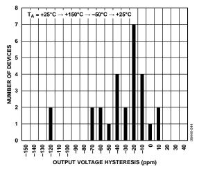
Figure 37. ADR3450 Thermally Induced Output Voltage Hysteresis Distribution
