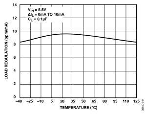
Figure 6. ADR3425 Load Regulation vs. Temperature (Sourcing)
