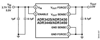
Figure 40. Basic Reference Connection
