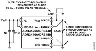
Figure 41. Application Showing Kelvin Connection
