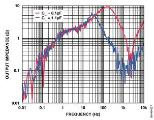
Figure 35. ADR3450 Output Impedance vs. Frequency
