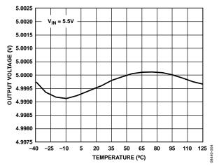
Figure 9. ADR3450 Output Voltage vs. Temperature
