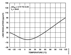
Figure 5. ADR3425 Line Regulation vs. Temperature
