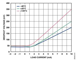
Figure 8. ADR3425 Dropout Voltage vs. Load Current
