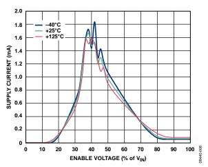
Figure 34. Supply Current vs. ENABLE Pin Voltage
