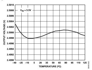
Figure 3. ADR3425 Output Voltage vs. Temperature
