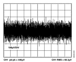
Figure 22. ADR3450 Output Voltage Noise (10 Hz to 10 kHz)
