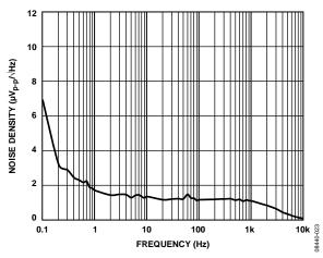
Figure 17. ADR3425 Output Noise Spectral Density
