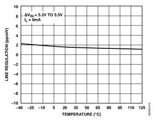
Figure 11. ADR3450 Line Regulation vs. Temperature
