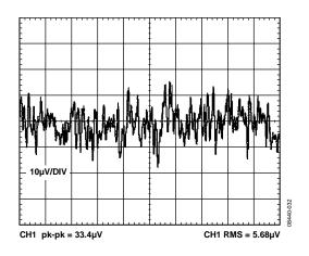
Figure 21. ADR3450 Output Voltage Noise (0.1 Hz to 10 Hz)
