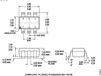
Figure 45. 6-Lead Small Outline Transistor Package (SOT-23) (RJ-6) Dimensions shown in millimeters
