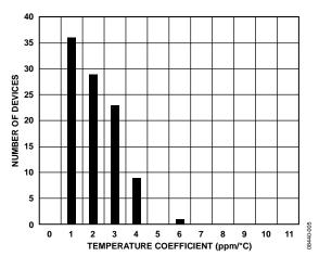
Figure 4. ADR3425 Temperature Coefficient Distribution
