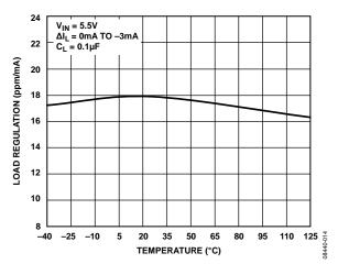
Figure 13. ADR3450 Load Regulation vs. Temperature (Sinking)
