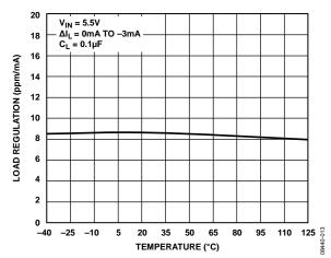
Figure 7. ADR3425 Load Regulation vs. Temperature (Sinking)
