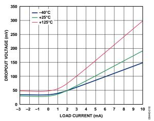
Figure 14. ADR3450 Dropout Voltage vs. Load Current
