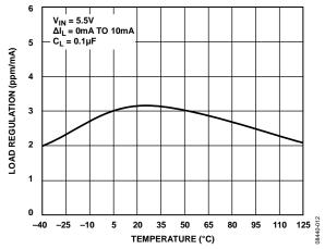
Figure 12. ADR3450 Load Regulation vs. Temperature (Sourcing)
