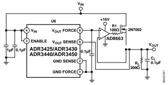
Figure 44. Boosted Output Current Reference
