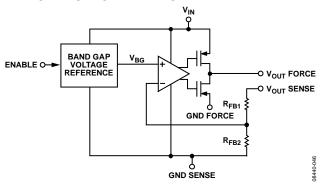
Figure 39. Block Diagram
