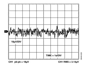
Figure 15. ADR3425 Output Voltage Noise (0.1 Hz to 10 Hz)
