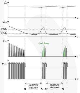
Figure 23. Burst-Mode Operation
