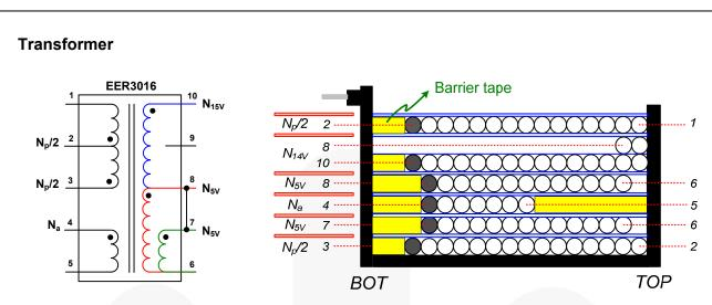
Figure 26. Schematic of Transformer
