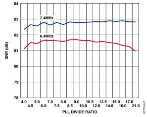
Figure 18. Single-Tone SNR vs. PLL Divide Ratio with  $f_{\rm IN1}=2.4$  MHz,  $f_{\rm IN2}=8.4$  MHz
