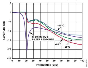
Figure 44. Maximum Input Level for 3 dB Noise Degradation
