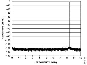
Figure 6. Single-Tone FFT with  $f_{IN} = 8.4 \text{ MHz}$
