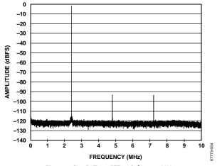
Figure 4. Single-Tone FFT with  $f_{IN} = 2.4 \text{ MHz}$
