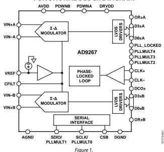
The AD9267 operates on a 1.8 V power supply, consuming 416 mW. The AD9267 is available in a 64-lead LFCSP and is specified over the industrial temperature range ( $-40^{\circ}$ C to  $+85^{\circ}$ C).
