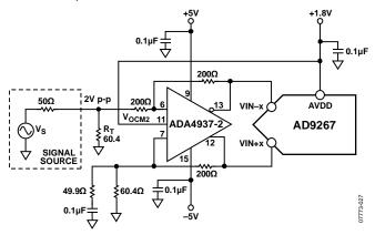
Figure 33. Differential Input Configuration Using the ADA4937-2
