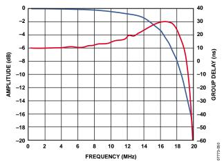
Figure 46. Low-Pass Chebyshev II Filter Response
