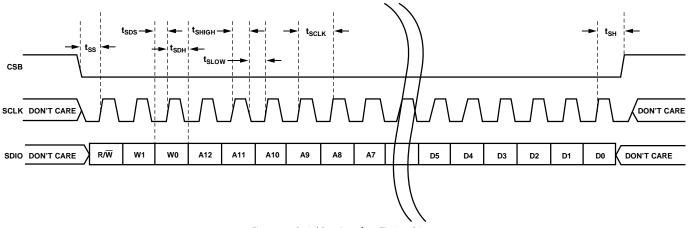
Figure 42. Serial Port Interface Timing Diagram
