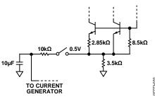
Figure 26. Equivalent VREF Circuit
