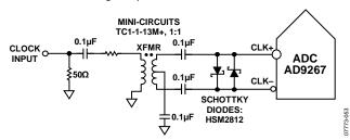
Figure 38. Transformer-Coupled Differential Clock
