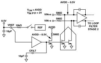
Figure 35. Voltage Reference Loop
