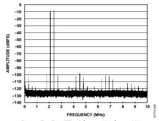
Figure 7. Two-Tone FFT with  $f_{IN1} = 2.1$  MHz,  $f_{IN2} = 2.4$  MHz
