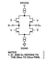
Figure 25. Equivalent Digital Output Circuit
