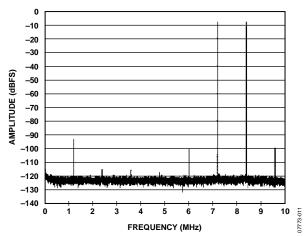
Figure 9. Two-Tone FFT with  $f_{IN1} = 7.2$  MHz,  $f_{IN2} = 8.4$  MHz
