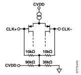
Figure 21. Equivalent Clock Input Circuit
