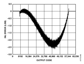
Figure 19. INL with  $f_{IN} = 2.4 \text{ MHz}$
