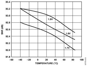
Figure 15. SNR vs. Temperature
