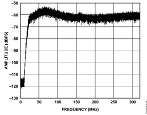
Figure 10. Noise Transfer Function (NTF)
