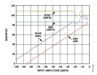
Figure 11. Single-Tone SNR and SFDR vs. Input Amplitude with  $f_{\rm IN}$  = 2.4 MHz
