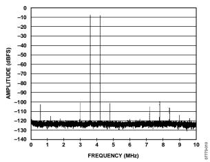
Figure 8. Two-Tone FFT with  $f_{IN1} = 3.6$  MHz,  $f_{IN2} = 4.2$  MHz
