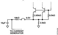
Figure 36. Internal Reference Configuration
