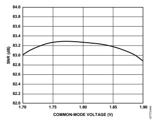
Figure 14. SNR vs. Input Common-Mode Voltage
