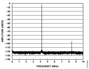
Figure 5. Single-Tone FFT with  $f_{IN} = 4.2 \text{ MHz}$
