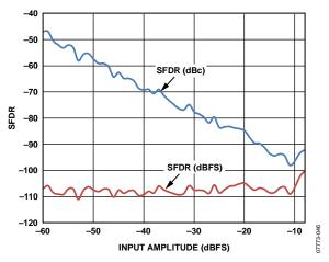
Figure 16. Two-Tone SFDR vs. Input Amplitude with  $f_{\rm IN1}=2.1$  MHz,  $f_{\rm IN2}=2.4$  MHz
