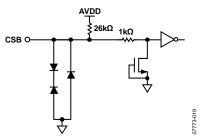
Figure 24. Equivalent CSB Input Circuit
