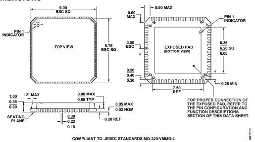
Figure 47. 64-Lead Lead Frame Chip Scale Package [LFCSP\_VQ] 9 mm × 9 mm Body, Very Thin Quad Dimensions shown in millimeters
