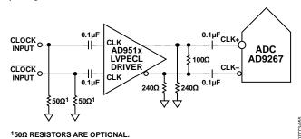
Figure 40. Differential LVPECL Sample Clock
