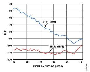
Figure 17. Two-Tone SFDR vs. Input Amplitude with  $f_{\rm IN1}=7.2$  MHz,  $f_{\rm IN2}=8.4$  MHz
