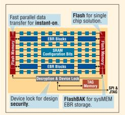
This approach provides a single chip solution, instant-on (1mS), FlashBAK EBR, TAG memory and design security.
