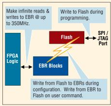
FlashBAK technology allows storage of multiple data types: error codes, data tables, and microprocessor code.
