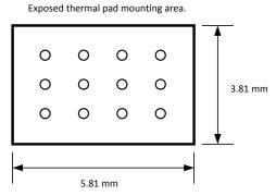
Vias are 0.3 mm diameter at 1.2 mm pitch. Recommended via plating of 1 oz copper.
