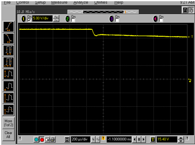
FIGURE 10. VLNb TRANSITIONS FROM 18.3V TO 13.3V
