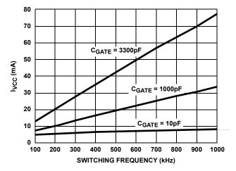
FIGURE 2. BIAS SUPPLY CURRENT vs FREQUENCY
