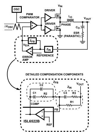
FIGURE 7. VOLTAGE - MODE BUCK CONVERTER COMPENSATION DESIGN
