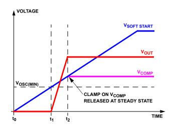
$$\begin{aligned} t_1 &= \frac{C_{SS}}{I_{SS}} \cdot V_{OSC(MIN)} \\ t_{SoftStart} &= t_2 - t_1 = \frac{C_{SS}}{I_{SS}} \cdot \frac{V_{OUT_{SteadyState}}}{V_{IN}} \cdot \Delta V_{OSC} \end{aligned}$$
