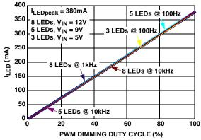
FIGURE 5. LEDs PWM DIMMING LINEARITY
