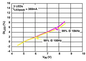
FIGURE 8. 3 LEDs CURRENT ACCURACY vs INPUT VOLTAGE
