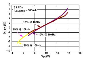
FIGURE 7. 5 LEDS CURRENT ACCURACY VS INPUT VOLTAGE
