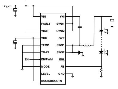
FIGURE 37. BASIC BUCK APPLICATION CIRCUIT
