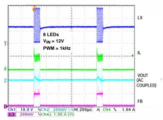
FIGURE 21. 10% PWM DIMMING AT 1kHz
