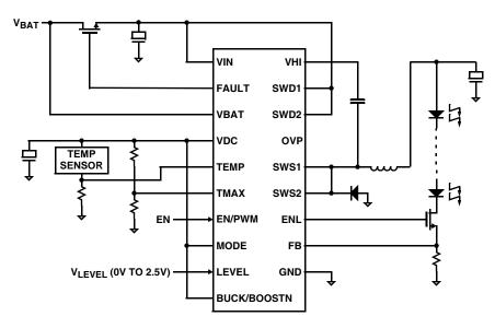
FIGURE 38. BUCK MODE WITH OVERCURRENT FAULT AND LED TEMPERATURE PROTECTIONS APPLICATION
