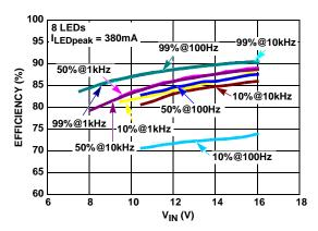
FIGURE 1. 8 LEDs EFFICIENCY vs INPUT VOLTAGE vs **DIMMING FREQUENCY AND DUTY CYCLE**
