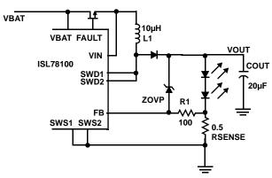
FIGURE 33. EXTERNAL OVP CIRCUIT
