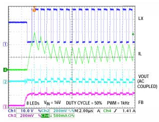
FIGURE 22. 50% PWM DIMMING AT 1kHz ZOOM-IN
