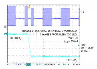
FIGURE 23. TRANSIENT RESPONSE OPERATES FROM 8 TO 7 LEDs
