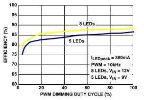
FIGURE 4. 8 AND 5 LEDs EFFICIENCY vs PWM DUTY CYCLE
