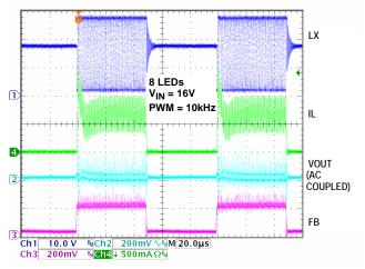
FIGURE 20. 50% PWM DIMMING AT 10kHz
