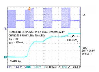
FIGURE 24. TRANSIENT RESPONSE OPERATES FROM 7 TO 8 LEDs
