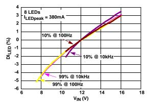
FIGURE 6. 8 LEDS CURRENT ACCURACY vs INPUT VOLTAGE
