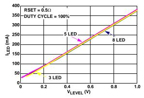
FIGURE 15. LED CURRENT vs V<sub>LEVEL</sub> BIAS
