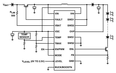
FIGURE 39. AUTOMOTIVE BOOST MODE APPLICATION DIAGRAM
