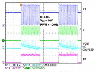
FIGURE 19. 50% PWM DIMMING AT 100Hz
