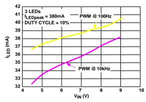
FIGURE 14. 3 LEDs LINE REGULATION OF PWM DUTY CYCLE OF 10%
