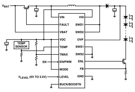
FIGURE 36. BOOST MODE APPLICATION WITH OVERCURRENT FAULT PROTECTION AND LED TEMPERATURE PROTECTION
