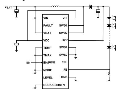
FIGURE 35. BASIC BOOST APPLICATION CIRCUIT
