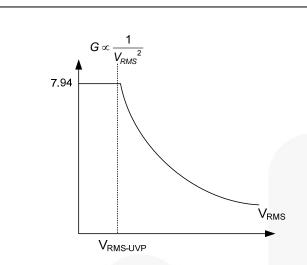
Figure 29. Modulation Gain Characteristics
