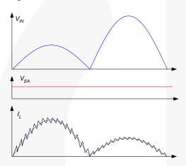
Figure 30. Line Feed-Forward Operation
