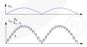
Figure 33. Inductor Current Shaping
