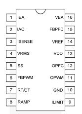
Figure 6. Pin Configuration (Top View)
