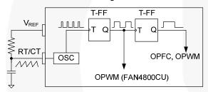
Figure 25. Oscillator Configuration
