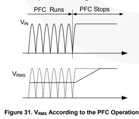
The rectified sinusoidal signal is obtained by the current flowing into the IAC pin. The resistor R<sub>IAC</sub> should be large enough to prevent saturation of the gain modulator, calculating as:
