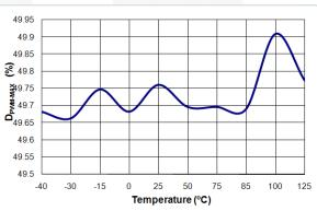
Figure 22. D<sub>PWM-MAX</sub> vs. Temperature
