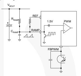
Figure 35. PWM Ramp Generation Circuit
