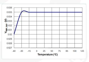
Figure 24. V<sub>RMS-SAG</sub> vs. Temperature
