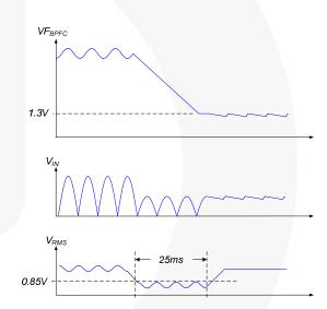
Figure 38. The Second condition of Sag Protection
