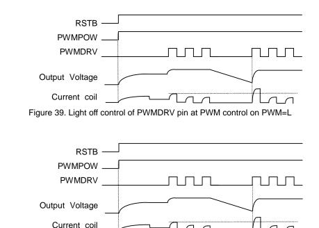
Figure 40. Light off control of PWMDRV pin at PWM control on RSTB=L
