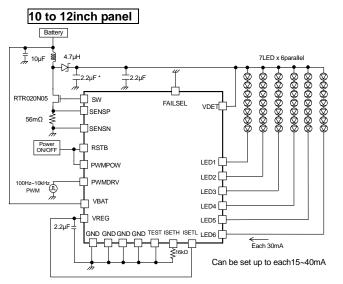
Figure 50. 7 series×6 parallel, LED current 30mA setting Current driver PWM application
