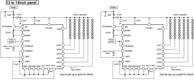
Figure 48. 8 series× 6 parallel, LED current 40mA setting Power control PWM application
