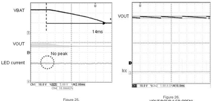
Figure 25. Line Transient (22V to 10V)
