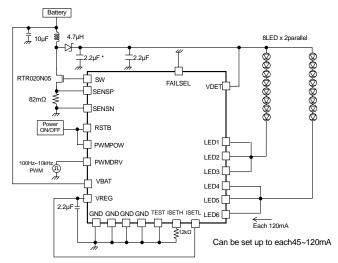
Figure 59. 8 series×2 parallel, LED current 120mA setting Current driver PWM application
