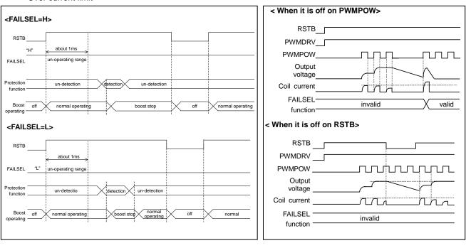
Figure 31. FAILSEL operating description
