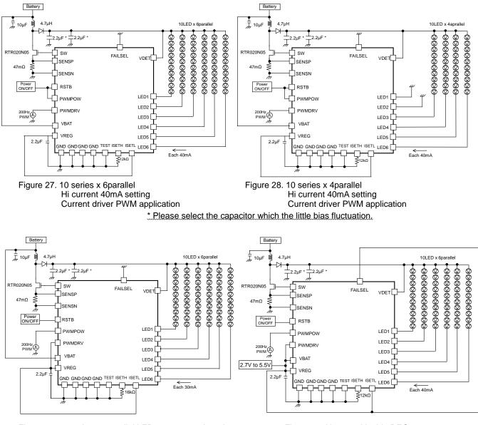
Figure 29. 10 series x 6parallel LED current 30mA setting Power control PWM application Figure 30. Non-used Inside REG or operating under 5V application
