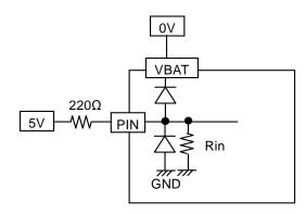
Figure 34. Voltage with a control sign higher than VBAT Example corresponding to application of conditions
