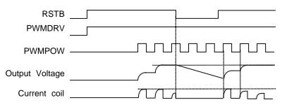
Figure 37. Light off control of PWMPOW pin at PWM control on RSTB=L
