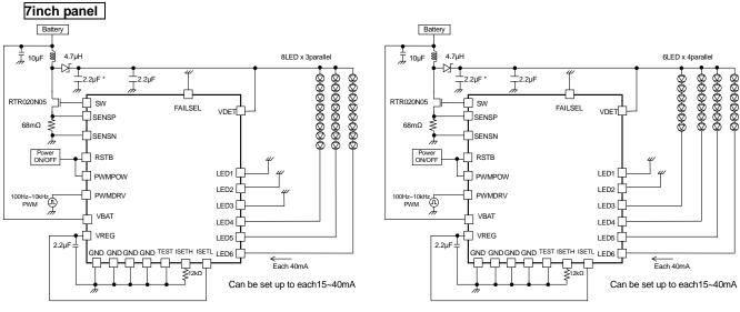
Figure 52. 8 series×3 parallel, LED current 40mA setting Current driver PWM application
