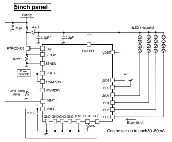
Figure 58. 4 series×4 parallel, LED current 40mA setting Current driver PWM application
