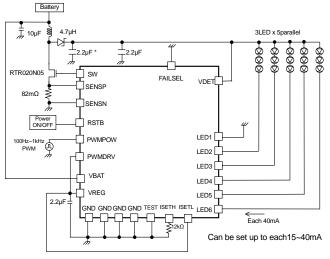
Figure 60. 3 series×5 parallel, LED current 40mA setting Power control PWM application
