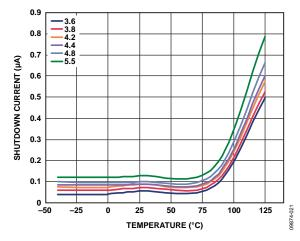
Figure 21. Shutdown Current vs. Temperature at Various Input Voltages
