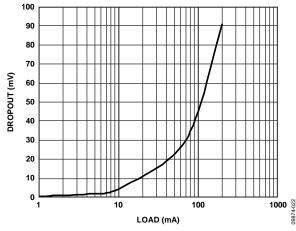
Figure 22. Dropout Voltage vs. Load Current and Output Voltage,  $V_{OUT1} = 3.3 V$
