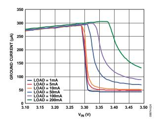
Figure 24. Ground Current vs. Input Voltage (in Dropout),  $V_{OUT1} = 3.3 V$
