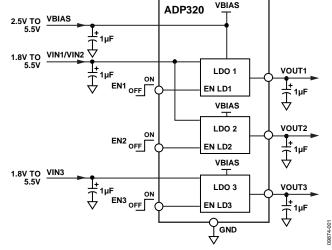
Figure 1. Typical Application Circuit
