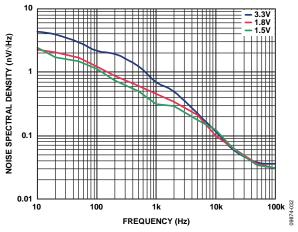
Figure 32. Output Noise Spectral Density,  $V_{IN} = 5 V$ ,  $I_{LOAD} = 10 \text{ mA}$
