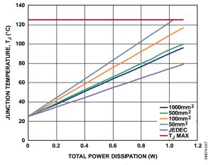
Figure 47. Junction Temperature vs. Total Power Dissipation,  $T_A = 25^{\circ}C$
