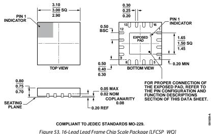
Figure 53. 16-Lead Lead Frame Chip Scale Package [LFCSP\_WQ] 3 mm × 3 mm Body, Very, Very Thin Quad (CP-16-27) Dimensions shown in millimeters
