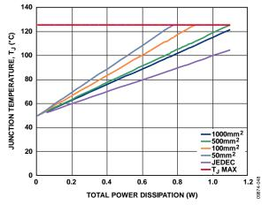
Figure 48. Junction Temperature vs. Total Power Dissipation,  $T_A = 50^{\circ}C$
