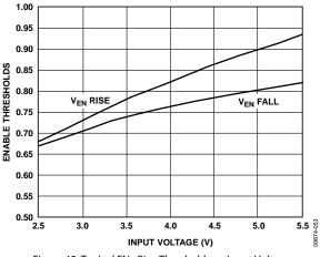
Figure 45. Typical ENx Pins Thresholds vs. Input Voltage
