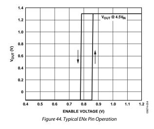
As shown in Figure 44, the ENx pin has built-in hysteresis. This prevents on/off oscillations that can occur due to noise on the ENx pin as it passes through the threshold points.
