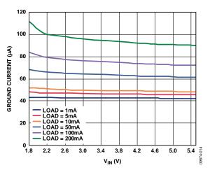
Figure 14. Ground Current vs. Input Voltage, Single Output Loaded
