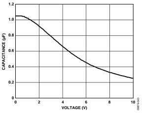
Figure 43. Capacitance vs. Voltage Bias Characteristic
