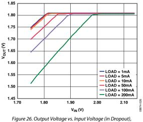
gure 26. Output Voltage vs. Input Voltage (in Dropout V<sub>OUT2</sub> = 1.8 V
