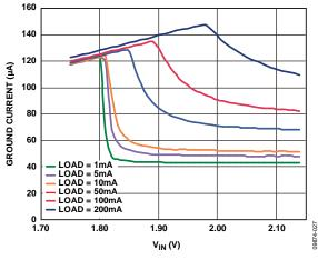
Figure 27. Ground Current vs. Input Voltage in Dropout),  $V_{OUT2} = 1.8 V$
