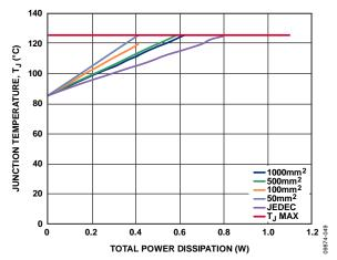
Figure 49. Junction Temperature vs. Total Power Dissipation,  $T_A = 85^{\circ}C$
