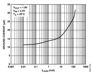
Figure 9. Ground Current vs. Load Current
