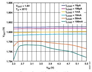
Figure 7. Output Voltage vs. Input Voltage
