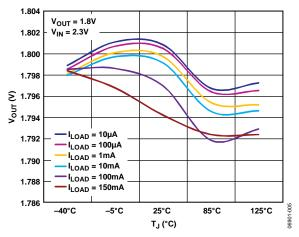
Figure 5. Output Voltage vs. Junction Temperature
