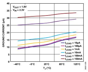
Figure 8. Ground Current vs. Junction Temperature
