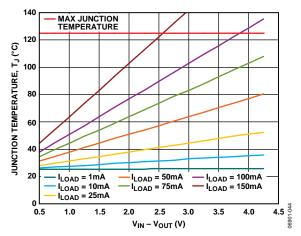
Figure 42. WLCSP, 0 mm<sup>2</sup> of PCB Copper,  $T_A = 25$ °C
