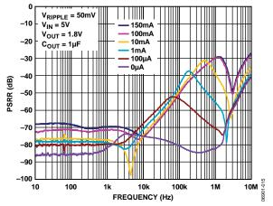
Figure 18. Power Supply Rejection Ratio vs. Frequency
