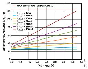
Figure 40. WLCSP, 500 mm<sup>2</sup> of PCB Copper,  $T_A = 25$ °C
