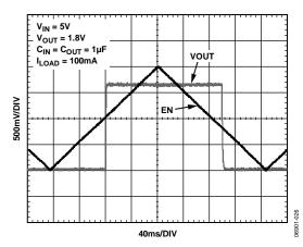
Figure 31. ADP121 Typical EN Pin Operation
