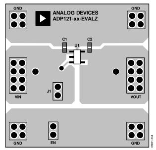
Figure 48. Example of TSOT PCB Layout
