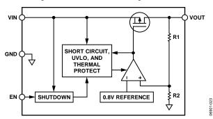
Figure 27. Internal Block Diagram
