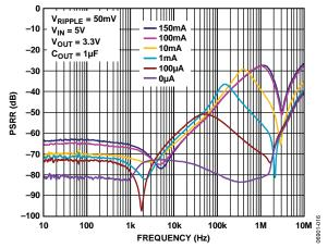
Figure 19. Power Supply Rejection Ratio vs. Frequency
