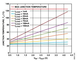
Figure 35. TSOT, 100 mm<sup>2</sup> of PCB Copper,  $T_A = 25$ °C
