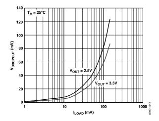
Figure 14. Dropout Voltage vs. Load Current, WLCSP
