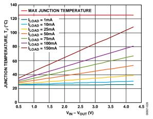
Figure 34. TSOT, 500 mm<sup>2</sup> of PCB Copper,  $T_A = 25$ °C
