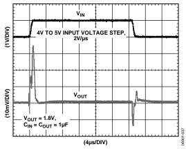
Figure 25. Line Transient Response, Load Current = 150 mA
