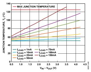
Figure 44. WLCSP, 100 mm<sup>2</sup> of PCB Copper,  $T_A = 50$ °C
