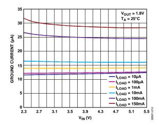
Figure 10. Ground Current vs. Input Voltage
