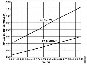
Figure 32. Typical EN Pin Thresholds vs. Input Voltage
