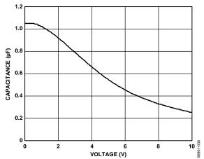
Figure 30. Capacitance vs. Voltage Bias Characteristic
