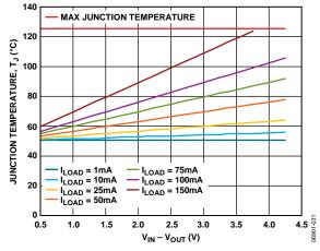
Figure 37. TSOT, 500 mm<sup>2</sup> of PCB Copper,  $T_A = 50$ °C
