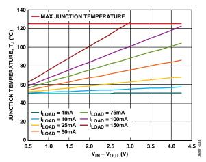
Figure 39. TSOT, 0 mm<sup>2</sup> of PCB Copper,  $T_A = 50^{\circ}$ C
