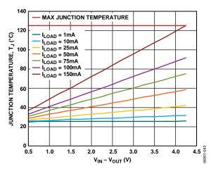
Figure 41. WLCSP, 100 mm<sup>2</sup> of PCB Copper,  $T_A = 25$ °C
