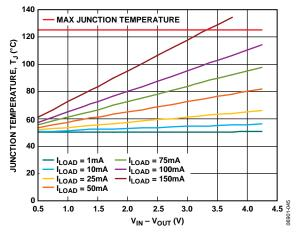
Figure 43. WLCSP, 500 mm<sup>2</sup> of PCB Copper,  $T_A = 50$ °C
