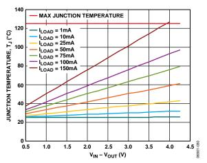
Figure 36. TSOT, 0 mm<sup>2</sup> of PCB Copper,  $T_A = 25$ °C
