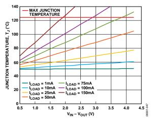
Figure 45. WLCSP, 0 mm<sup>2</sup> of PCB Copper,  $T_A = 50$ °C
