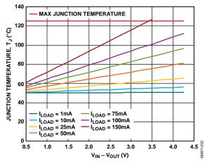
Figure 38. TSOT, 100 mm<sup>2</sup> of PCB Copper,  $T_A = 50$ °C
