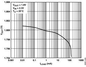
Figure 6. Output Voltage vs. Load Current
