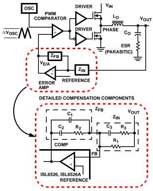
FIGURE 5. VOLTAGE-MODE BUCK CONVERTER COMPENSATION DESIGN
