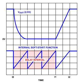
FIGURE 3. OVERCURRENT PROTECTION RESPONSE
