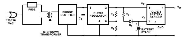
FIGURE 9. POWER SUPPLY FOR LOW POWER PORTABLE AC TO DC SYSTEMS
