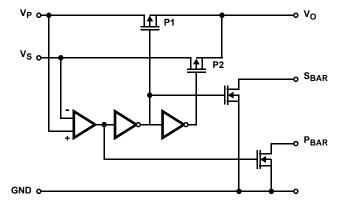
$V_P > V_S$ , P1 SWITCH ON AND PBAR SWITCH ON  $V_S > V_P$ , P2 SWITCH ON AND SBAR SWITCH ON
