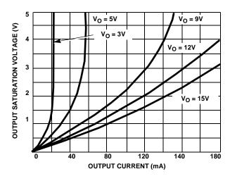
FIGURE 4. PBAR OR SBAR SATURATION VOLTAGE AS A FUNCTION OF OUTPUT CURRENT
