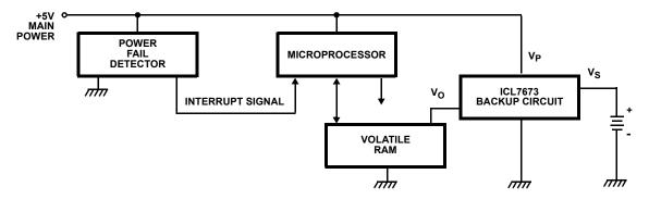
FIGURE 10. TYPICAL MICROPROCESSOR MEMORY APPLICATION
