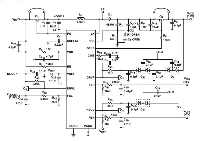
NOTE: SGND should be connected to PGND at one point only.
