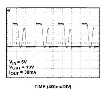
FIGURE 17. LX WAVEFORM - DISCONTINUOUS MODE
