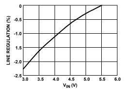
FIGURE 10. V<sub>BOOST</sub> LINE REGULATION (P-MODE)
