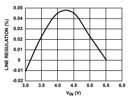
FIGURE 9. VBOOST LINE REGULATION (PI-MODE)
