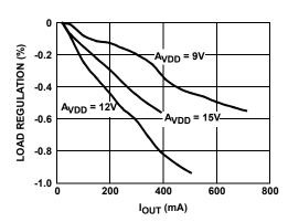
FIGURE 6. V<sub>BOOST</sub> LOAD REGULATION AT V<sub>IN</sub> = 5V (PI-MODE)
